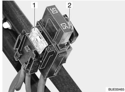
Fig. 196 Fuses on the starter battery
