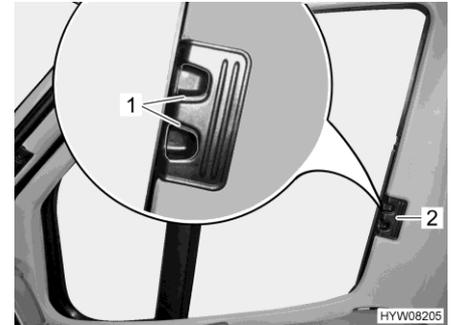
Fig. 42 Roman shade for the driver's / front passenger's window
