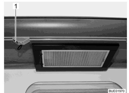
Fig. 249 Recirculating extractor hood
