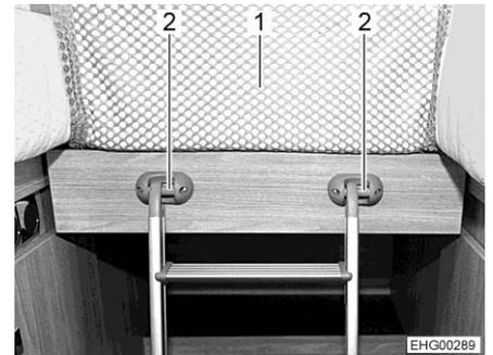
Fig. 172 Access ladder and safety net
