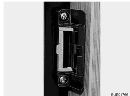
Fig. 266 Locking device in ventilation position
