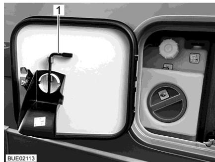
Fig. 282 Service flap with square spanner
