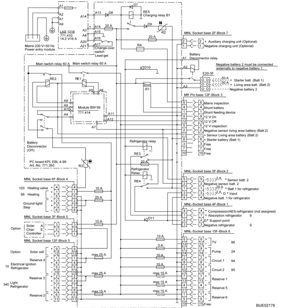
Fig. 211 Circuit diagram, interior (EBL 119)
