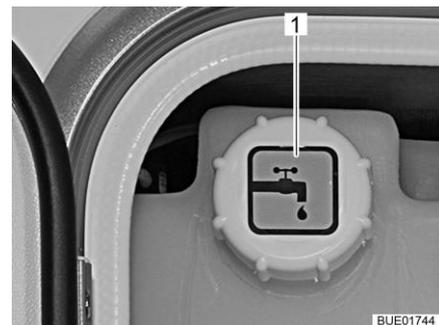
Fig. 268 Drinking water filler neck in service unit (alternative)
