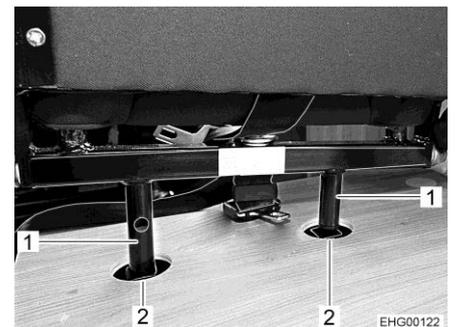
Fig. 31 Bars (inserted)
