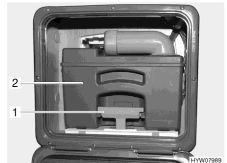
Fig. 300 Sewage tank (example)
