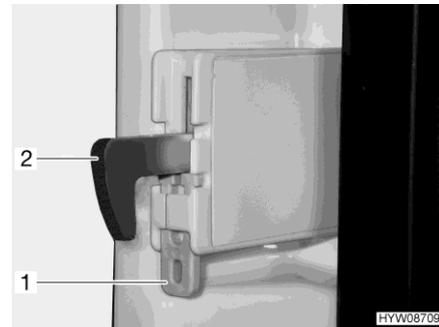
Fig. 259 Fixture (lock hook)
