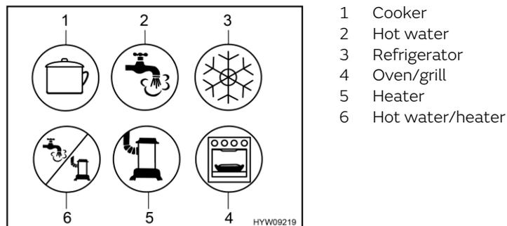
Fig. 216 Possible symbols for the gas isolator taps
