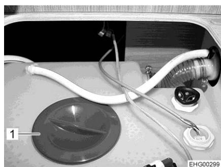
Fig. 302 Cleaning opening of the water tank
