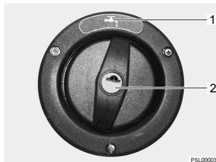
Fig. 267 Drinking water filler neck in the vehicle's side wall
