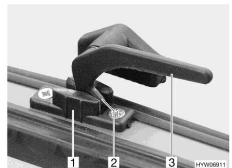
Fig. 98 Catch lever in "continuous ventilation" position
