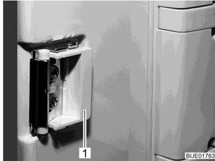
Fig. 263 Locking device in normal position
