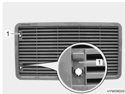
Fig. 250 Refrigerator ventilation grill (with sliding trap)
