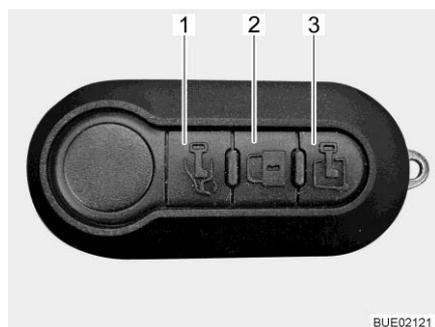
Fig. 51 Multifunctional remote control (3 buttons)
