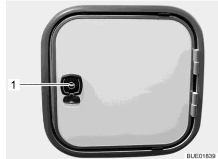
Fig. 286 Flap for sewage tank (alternative)
