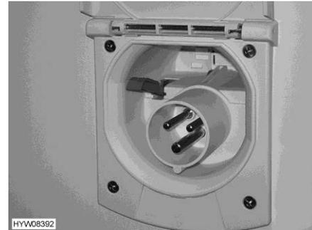
Fig. 194 230 V connection on the vehicle (without service unit)
