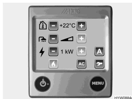
Fig. 224 Adjustment menu (operating unit)
