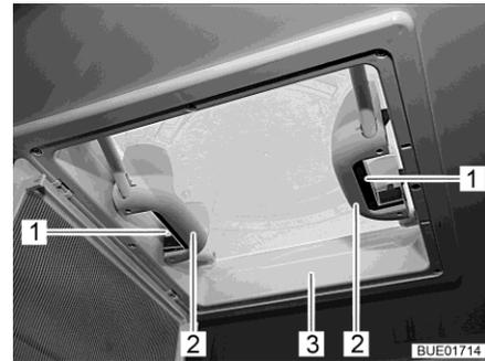
Fig. 109 Handles with snap latches
