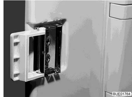
Fig. 264 Locking device in ventilation position
