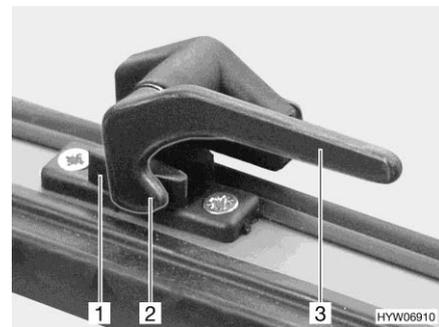
Fig. 94 Catch lever in "closed" position
