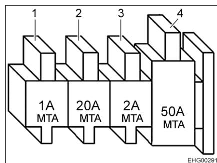
Fig. 198 Fuses (living area battery with charging booster)
