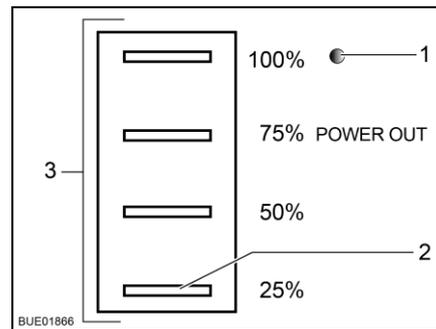
Fig. 190 Status indicator, solar charge regulator
