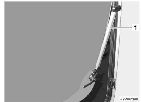
Fig. 96 Hinged window with automatic hinge
