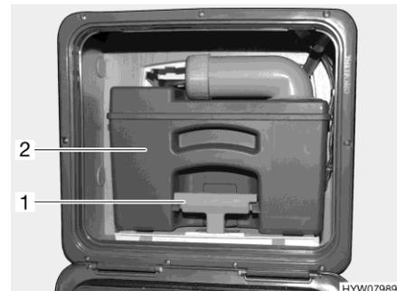
Fig. 288 Sewage tank (example)
