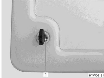
Fig. 59 Service flap push-button lock
