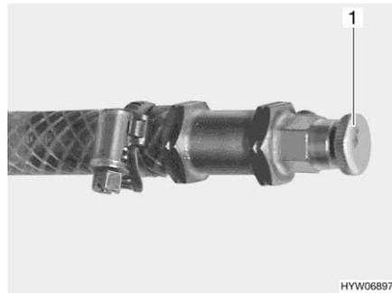
Fig. 306 Bleeding valve of hot-water heater
