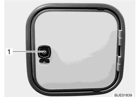
Fig. 298 Flap for the sewage tank (alternative)
