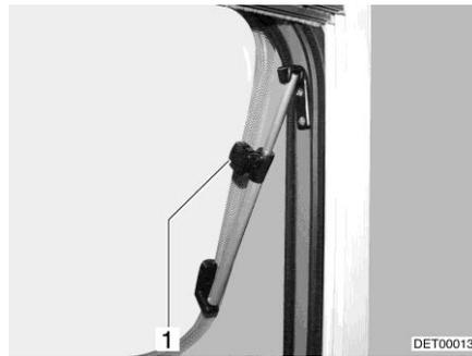
Fig. 95 Hinged window with rotary hinge
