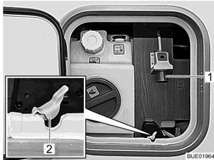
Fig. 193 230 V connection on the vehicle (with service unit)
