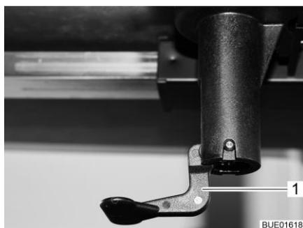
Fig. 124 Unlocking of the table top
