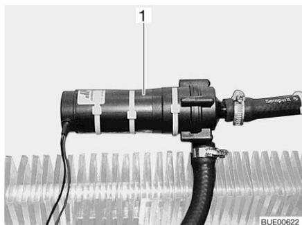
Fig. 228 Auxiliary circulating pump
