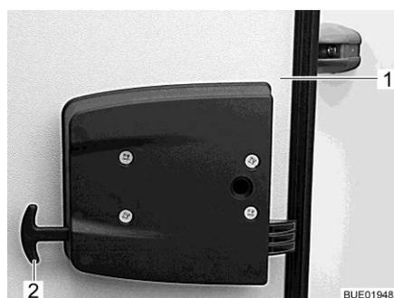
Fig. 58 Garage flap emergency release
