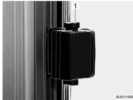
Fig. 99 Sliding window, locked
