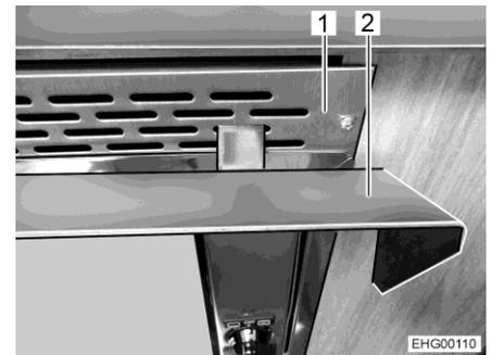
Fig. 244 Heat protection sheet (hooked in)
