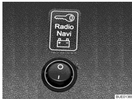
Fig. 185 Selector switch for power supply
