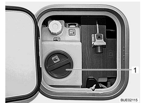
Afb. 281 Reinigingsopening watertank (service-unit)
