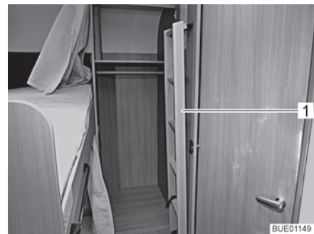
Fig. 12 Access ladder in the wardrobe
