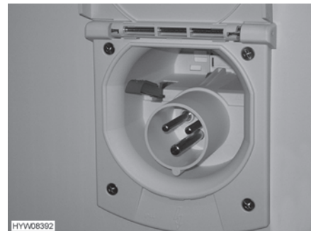
Fig. 122 230 V connection on vehicle
