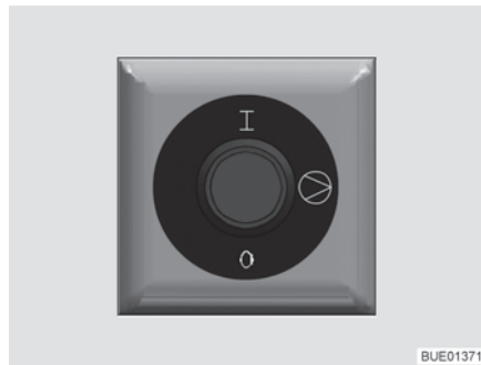
Fig. 142 Operating switch for auxiliary circulating pump
