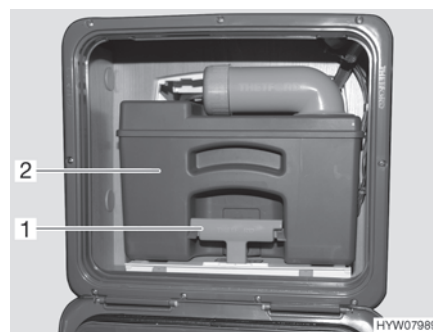
Fig. 175 Sewage tank (example)
