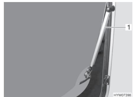
Fig. 96 Hinged window with automatic hinge
