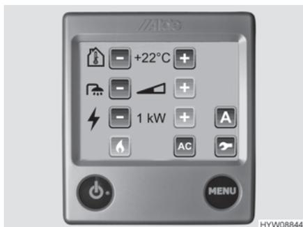
Fig. 157 Adjustment menu (operating unit)
