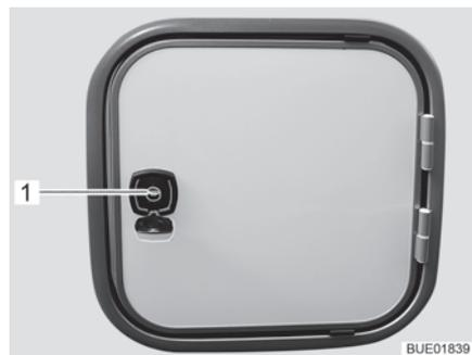
Fig. 200 Flap for sewage tank
