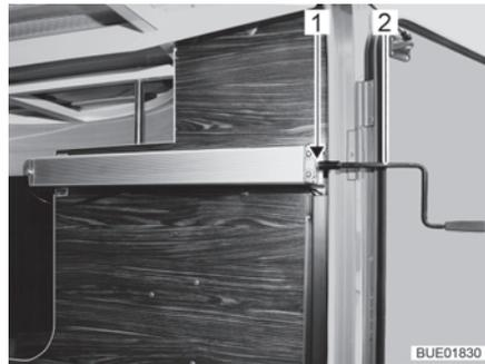
Fig. 124 Crank in the rear garage
