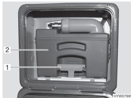
Fig. 209 Sewage tank (example)
