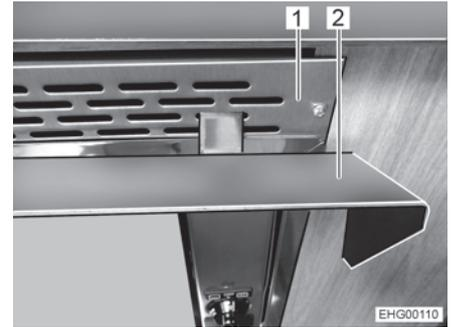
Fig. 175 Heat protection sheet (hooked in)
