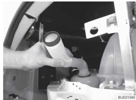
Fig. 43 Filler neck in filling position
