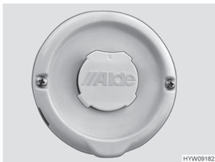
Fig. 164 Wall flue of the hot-water heater
