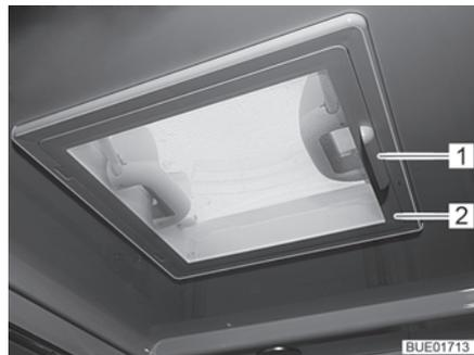
Fig. 111 Skylight with snap latch
