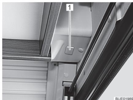
Fig. 105 Access to emergency operation
