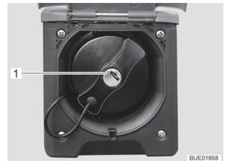
Fig. 45 Cap for the fuel filler neck
