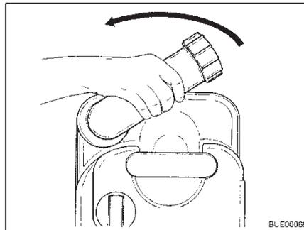
Fig. 202 Turning drainage neck
