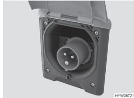
Fig. 142 230 V connection on vehicle
