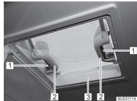
Fig. 112 Handles with snap latches
