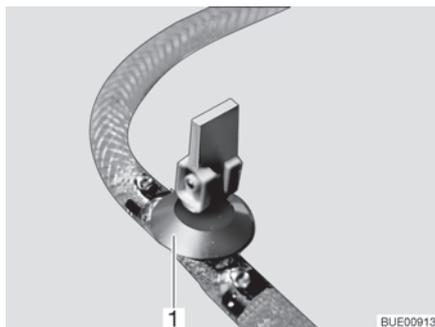
Fig. 194 Drain cock (with rocking lever)
