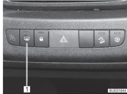
Fig. 35 External mirror heater switch
