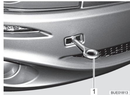
Fig. 47 Towing eye, mounted
