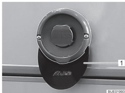
Fig. 13 Flue shield
