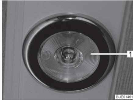
Fig. 84 Recessed light, light switch in the lamp
