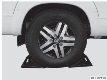
Fig. 228 Securing vehicle
