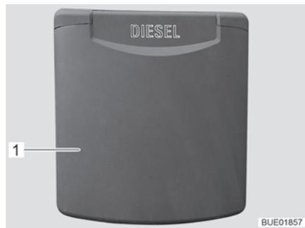
Fig. 44 Fuel filler neck external flap
