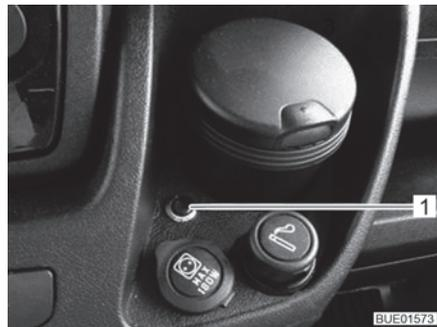
Fig. 50 Push-button to activate remote control
