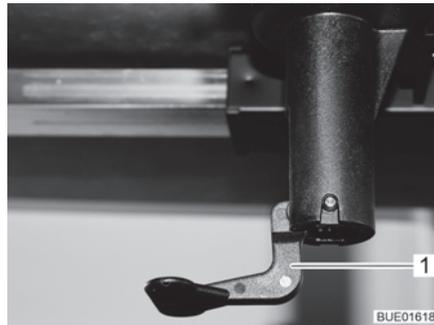
Fig. 116 Unlocking of the table top
