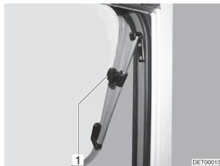
Fig. 95 Hinged window with rotary hinge
