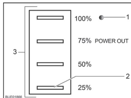
Fig. 140 Status indicator, solar charge regulator
