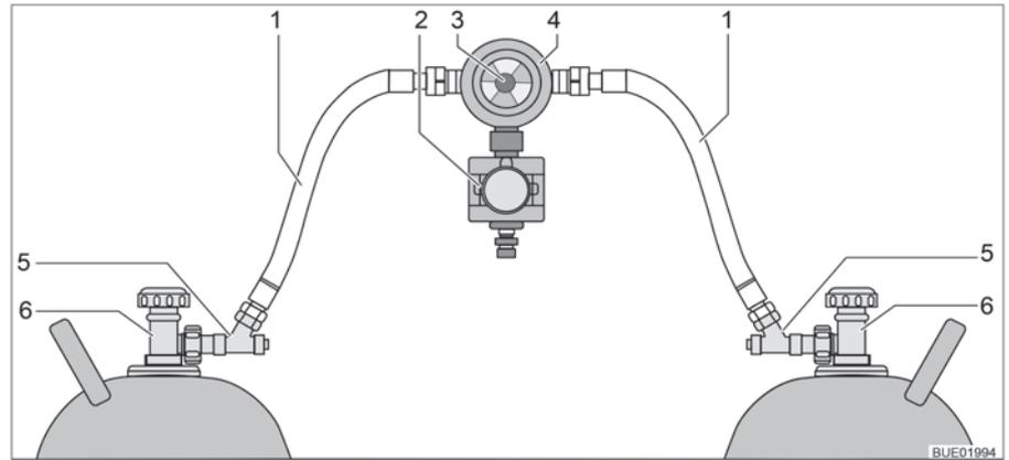
Fig. 22 Gas regulator with CPU and hose break guard
