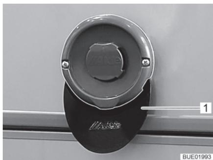
Fig. 165 Flue shield
