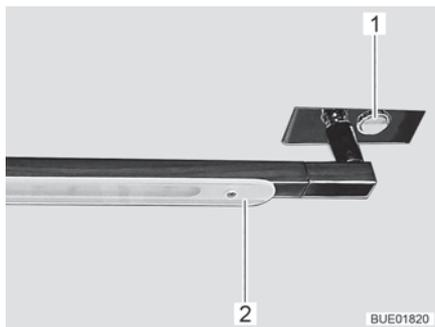
Fig. 82 Tube lamp, swivelling
