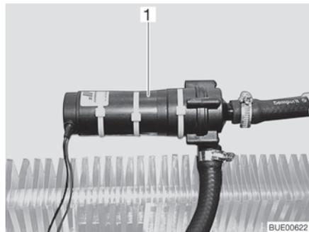
Fig. 161 Auxiliary circulating pump
