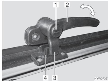
Fig. 93 Catch lever with safety knob in "closed" position
