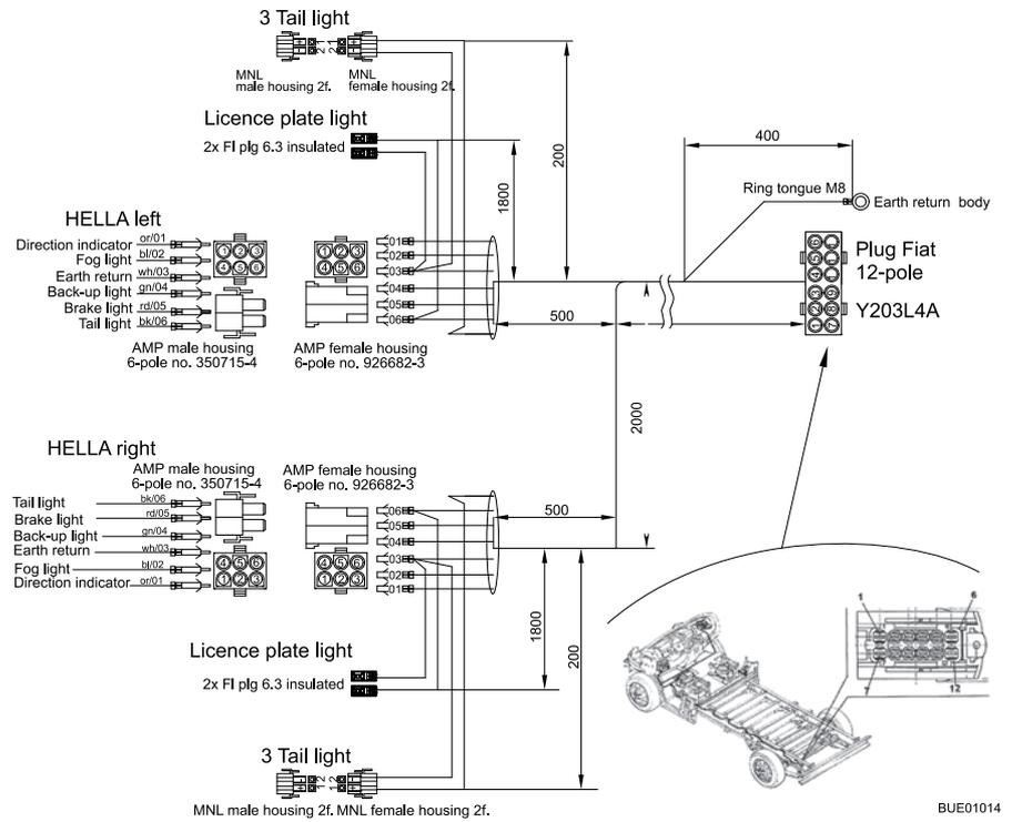
Fig. 153 Circuit diagram, exterior
