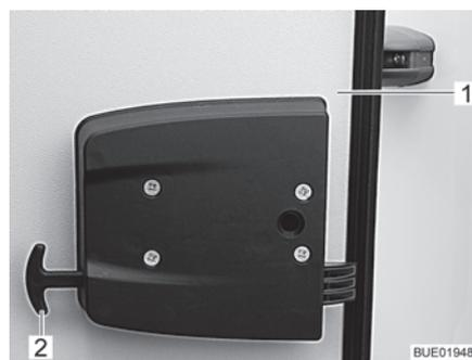
Fig. 67 Garage flap emergency release
