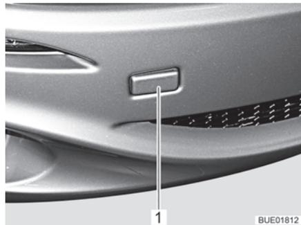
Fig. 46 Cover for the towing eye holder (example)
