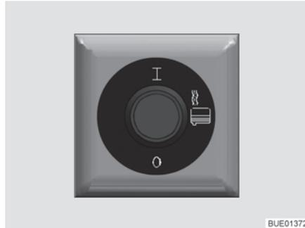
Fig. 198 Switch for waste water heating
