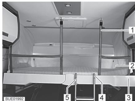
Fig. 120 Pull-down bed complete with applied safety net
