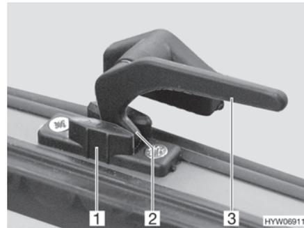
Fig. 98 Catch lever in "continuous ventilation" position
