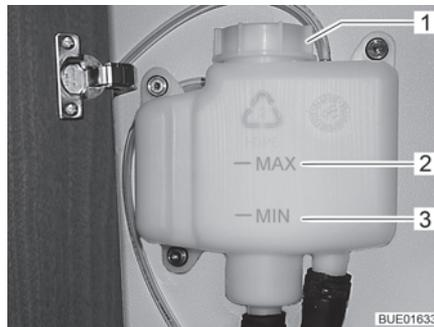
Fig. 212 Compensator reservoir without panel
