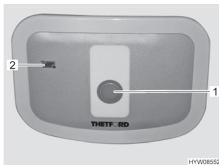
Fig. 207 Flush button/indicator lamp Thetford toilet (alternative)
