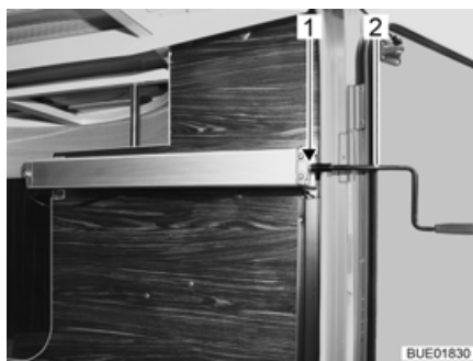
Afb. 124 Handslinger in garage achter
