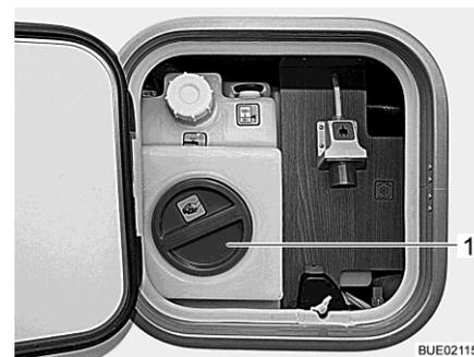
Fig. 278 Cleaning opening of the water tank (service unit)
