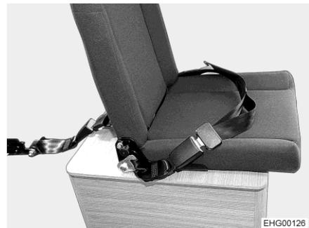
Fig. 36 Seat (completely fitted)
