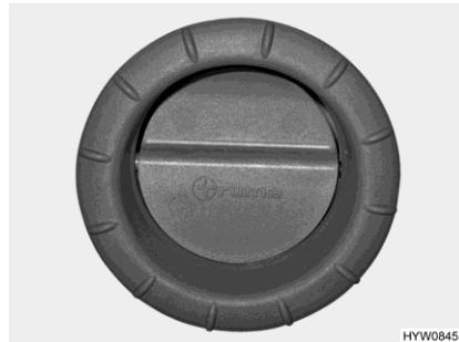
Fig. 204 Air outlet nozzle (hot-air heater)
