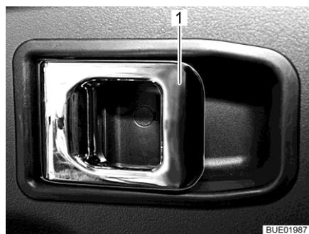
Fig. 71 Door lock (driver's door, inside)
