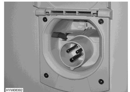
Fig. 189 230 V connection on the vehicle
