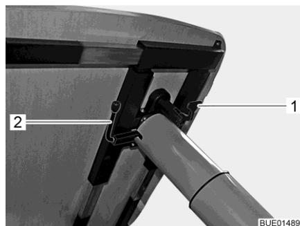
Fig. 130 Adjustment of lift-off table
