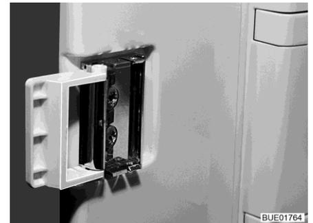
Fig. 245 Locking device in ventilation position
