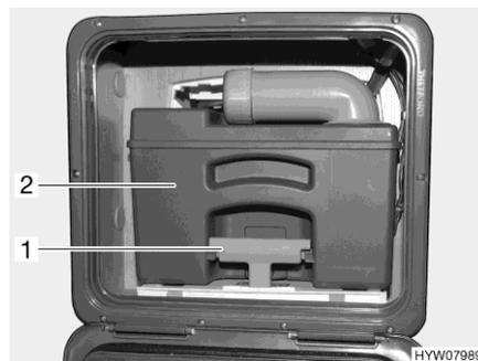
Fig. 275 Sewage tank (example)
