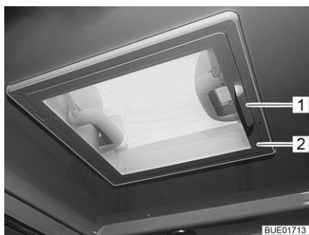
Fig. 124 Skylight with snap latch
