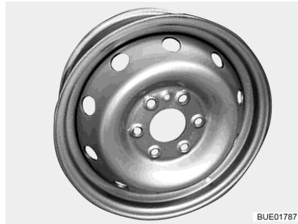
Fig. 299 Steel wheel rim (standard)
