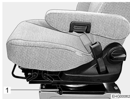
Fig. 24 Release lever for rotating
