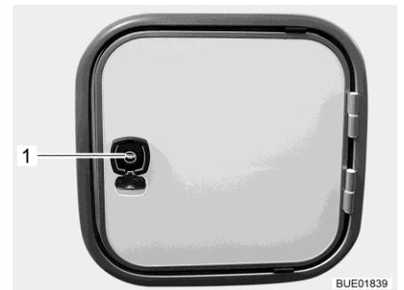
Fig. 265 Flap for sewage tank (alternative)
