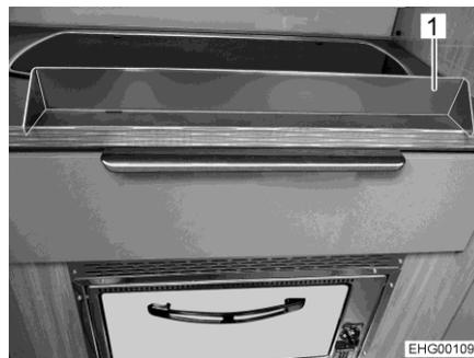
Fig. 229 Heat protection sheet (loose)
