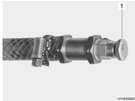
Fig. 281 Bleeding valve of hot-water heater
