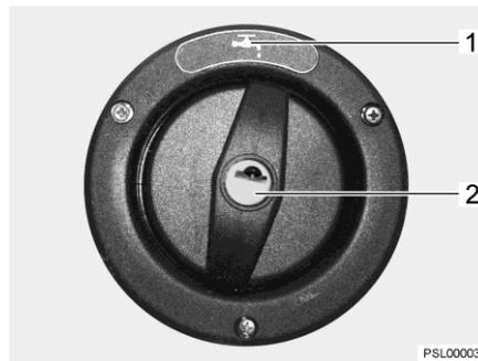
Fig. 85 Cap for the drinking water filler neck
