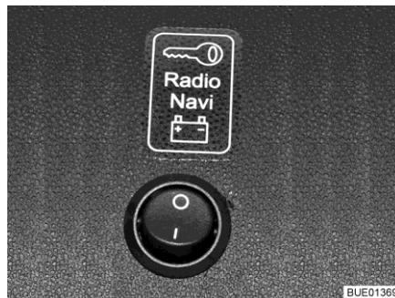
Fig. 178 Selector switch for operating behaviour
