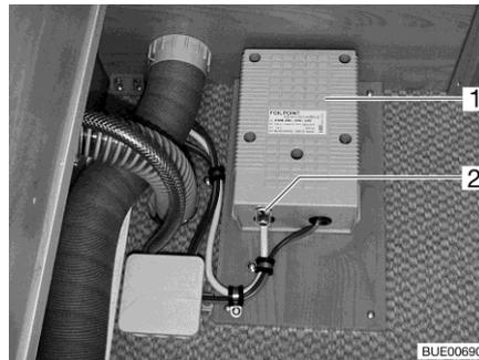
Fig. 220 Transformer for electrical floor warming unit
