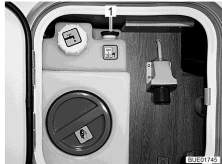
Fig. 255 Water tank with rotary handle in service unit
