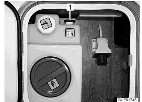
Fig. 253 Water tank with rotary handle in service unit
