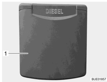
Fig. 56 Fuel filler neck external flap
