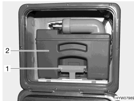
Fig. 266 Sewage tank (example)
