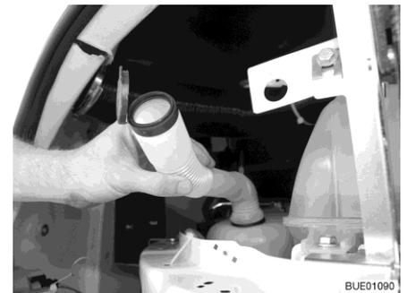
Fig. 55 Filler neck in filling position
