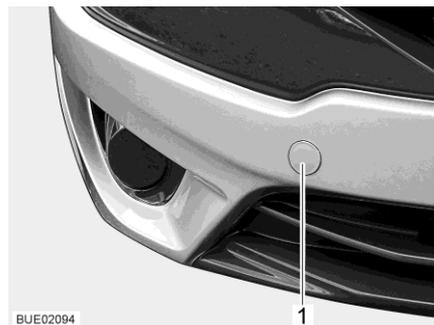
Fig. 59 Cover for the towing eye holder (example)
