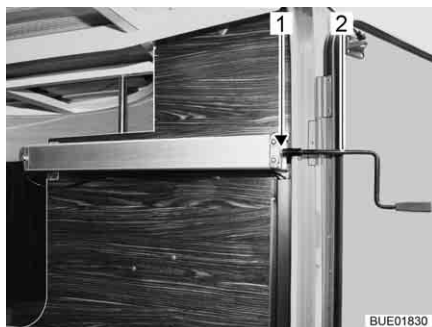
Afb. 147 Handslinger in garage achter
