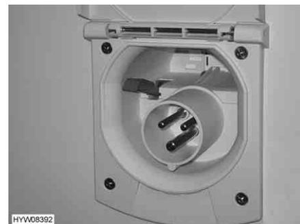
Fig. 101 230 V connection on vehicle
