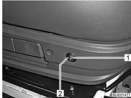
Fig. 14 Switch for seat heater
