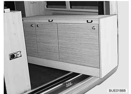
Fig. 86 Removing the sideboard
