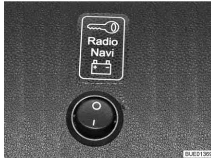
Fig. 96 Selector switch for operating behaviour
