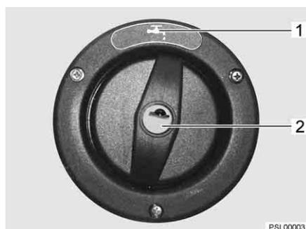
Fig. 140 Cap for the drinking water filler neck
