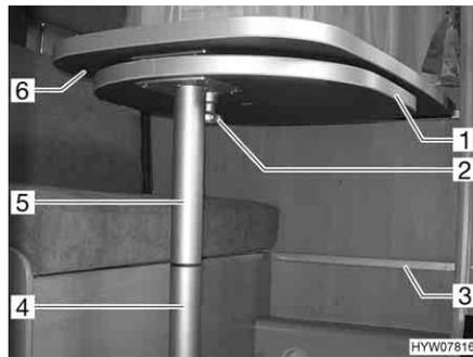
Fig. 70 Suspension table with separable support leg
