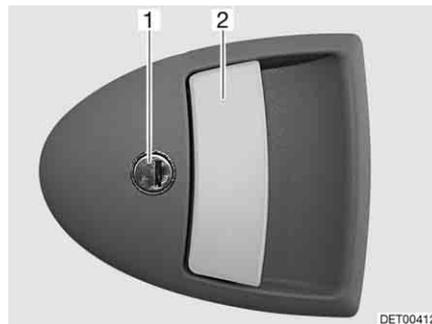
Fig. 28 Door lock of conversion door, outside
