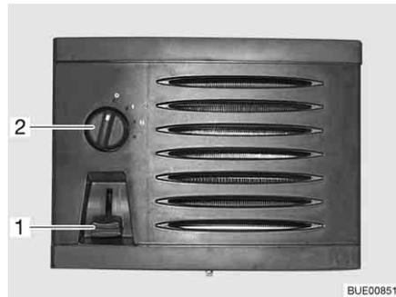
Fig. 120 Operating controls for auxiliary heat exchanger
