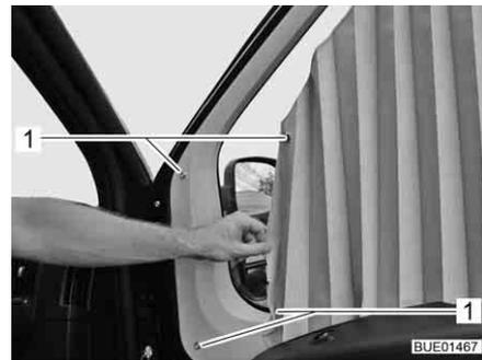
Fig. 55 Fixing of pleated shades
