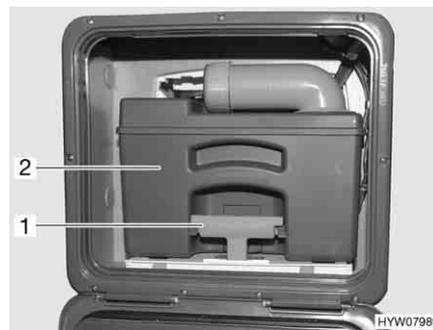
Fig. 152 Sewage tank (example)
