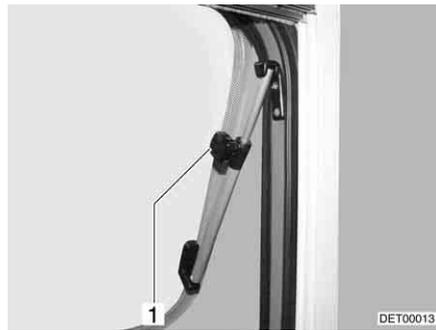
Fig. 49 Hinged window with rotary hinge
