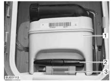
Fig. 164 Flap for sewage tank
