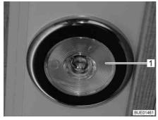
Fig. 46 Recessed light, light switch in the lamp
