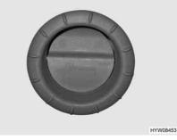
Fig. 126 Air outlet nozzle of the hot air distribution
