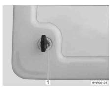
Fig. 37 Push-button lock service flap
