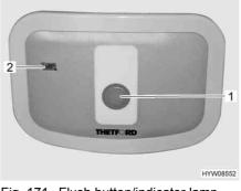
Fig. 170 Flush button/indicator lamp Thetford toilet
