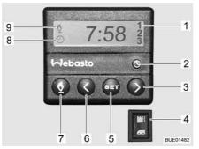
Fig. 135 Operating unit for independent vehicle heater
