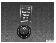
Fig. 103 Selector switch for operating behaviour
