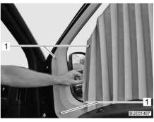
Fig. 63 Fixing of pleated shades
