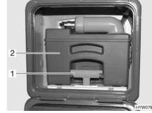
Fig. 176 Flap for the sewage tank
