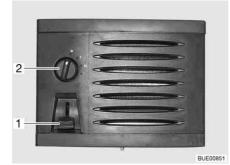
Fig. 132 Operating controls for auxiliary heat exchanger
