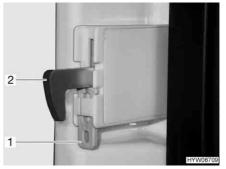
Fig. 149 Release button of the refrigerator door (Dometic 8 series)
