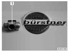
Fig. 11 Reversing camera with infrared illumination
