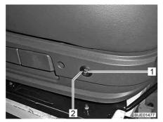
Fig. 14 Switch for seat heater
