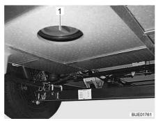
Fig. 178 Cleaning opening on the waste water tank
