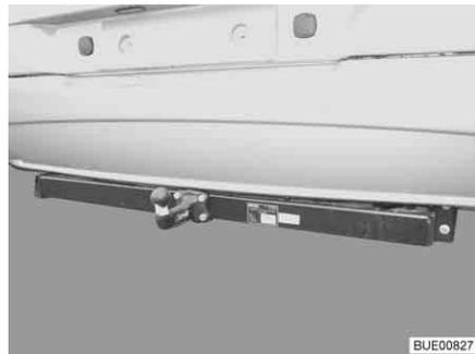
Fig. 10 Engate do reboque
