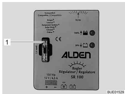
Fig. 182 Solar charge regulator fuse 100 W
