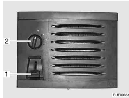
Fig. 204 Operating controls for auxiliary heat exchanger
