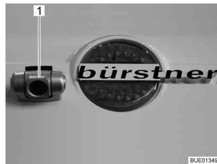
Fig. 22 Reversing camera with infrared illumination (Waeco)
