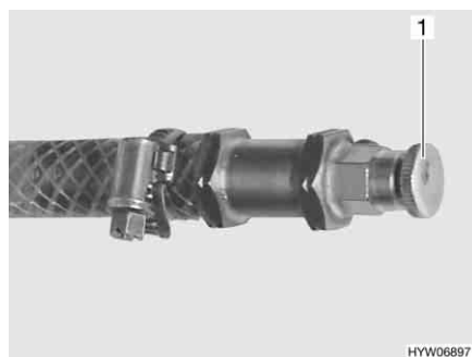
Fig. 265 Bleeding valve of hot-water heater
