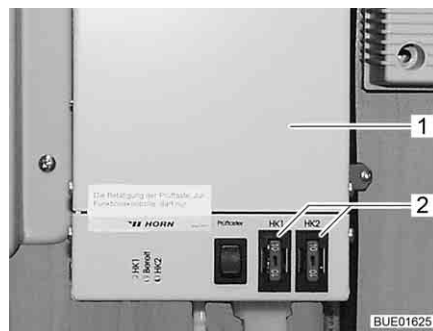
Fig. 168 Heater regulation for waste water pipes
