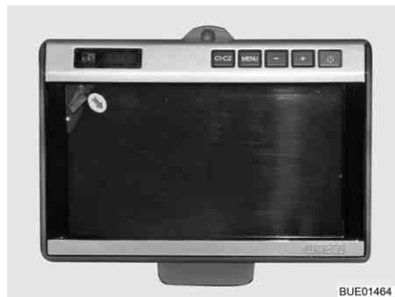
Fig. 19 LCD monitor for reversing camera (Waeco)
