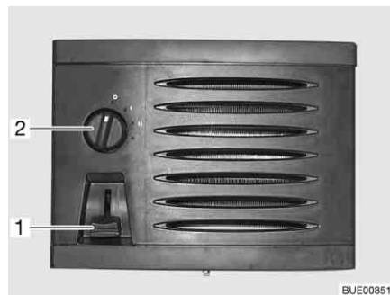
Fig. 194 Operating controls for auxiliary heat exchanger
