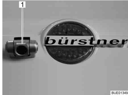
Fig. 17 Reversing camera with infrared illumination (Waeco)
