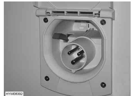
Fig. 140 230 V connection on vehicle
