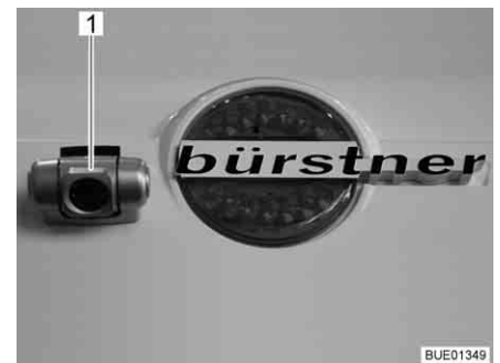
Fig. 22 Reversing camera with infrared illumination (Waeco)
