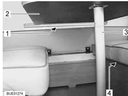
Fig. 104 Suspension table with changeable table leg
