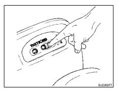
Fig. 254 Closing the sliding trap
