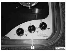
Fig. 212 Operating controls for gas cooker
