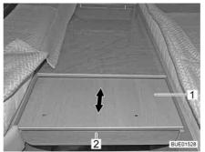
Fig. 137 Pull out bed widening
