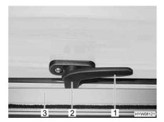
Fig. 99 Catch lever in "closed" position
