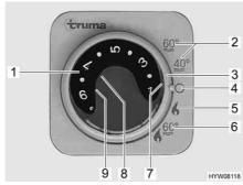
Fig. 189 Operating unit for heater/boiler
