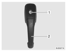
Fig. 56 Door lock of conversion door, outside
