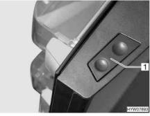
Fig. 225 Release button of the refrigerator door (Dometic 8 series)
