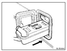
Fig. 264 Inserting the Thetford cassette
