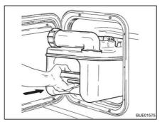
Fig. 247 Inserting the Thetford cassette
