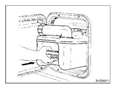
Fig. 272 Inserting the Thetford cassette
