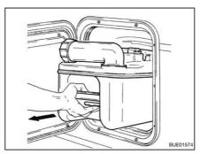
Fig. 244 Removing the Thetford cassette
