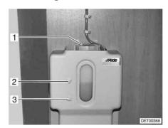
Fig. 281 Compensator reservoir hotwater heater
