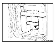
Fig. 243 Pulling the retaining clip
