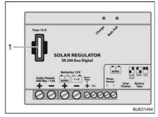
Fig. 175 Solar charge regulator fuse 200 W
