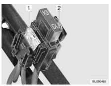
Fig. 168 Fuses on the starter battery
