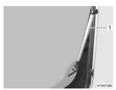
Fig. 95 Hinged window with automatic hinges
