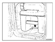
Fig. 260 Pulling the retaining clip
