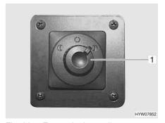
Fig. 32 External mirror adjustment switch
