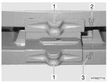
Fig. 223 Locking of the refrigerator door/freezer compartment door (Dometic 7 series with separate freezer compartment)
