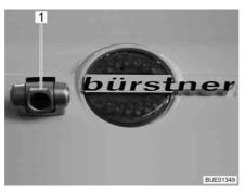
Fig. 16 Reversing camera with infrared illumination (Waeco)
