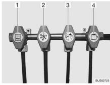
Fig. 187 Symbols for the gas isolator taps
