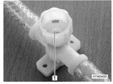
Fig. 241 Drain cock (with rocking lever)
