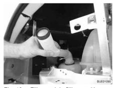
Fig. 43 Filler neck in filling position
