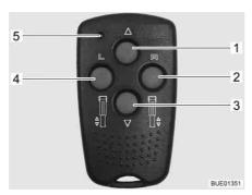
Fig. 47 Remote control for electrical steady legs
