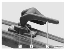
Fig. 92 Catch lever in the "continuous ventilation" position
