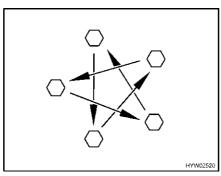
Fig. 306 Tighten the wheel nuts or wheel bolts cross-wise
