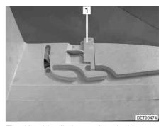
Fig. 107 Ventilation position locking mechanism
