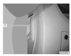
Fig. 40 Release lever for the bonnet (inside the vehicle)
