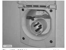
Fig. 166 230 V connection on vehicle
