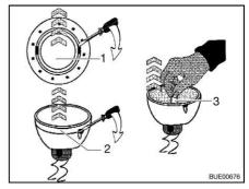
Fig. 297 Recessed halogen light (flat)
