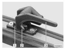
Fig. 89 Catch lever in "closed" position
