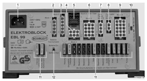
Fig. 154 Transformer/rectifier (EBL 99)
