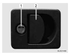
Fig. 62 Flap lock with recessed handle
