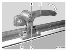
Fig. 96 Catch lever with safety knob in "continuous ventilation" posi-
