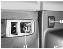
Fig. 31 External mirror adjustment and heater switch
