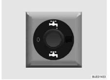
Fig. 237 Operating switch for electrically operated drainage valve (special equipment)
