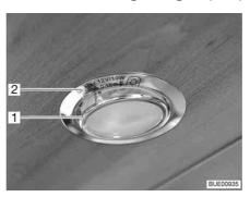
Fig. 299 Recessed halogen light (flat)
