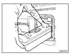
Fig. 261 Removing the Thetford cassette
