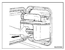
Fig. 269 Removing the Thetford cassette
