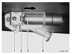
Fig. 49 Electrical steady leg on vehicle
