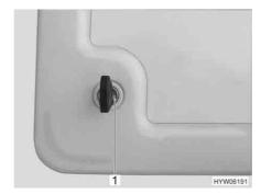
Fig. 64 Push-button lock service flap
