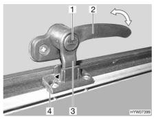
Fig. 91 Catch lever with safety knob in "continuous ventilation" posi-
