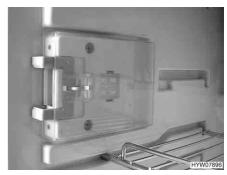
Fig. 228 Locking device in ventilation position
