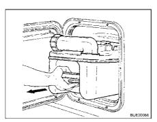
Fig. 256 Removing the Thetford cas-
