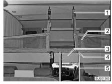
Fig. 125 Pull-down bed complete with applied safety net
