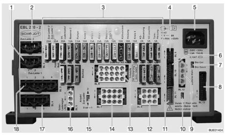
Fig. 155 Transformer/rectifier (EBL 220)
