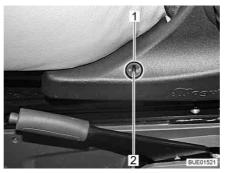
Fig. 24 Seat heater switch
