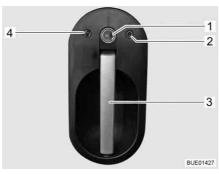
Fig. 54 Door lock of driver's door, outside
