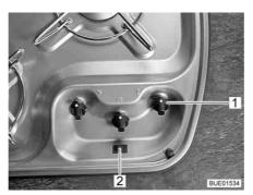
Fig. 211 Operating controls for gas cooker
