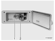
Fig. 148 External gas connection, gas isolator tap closed
