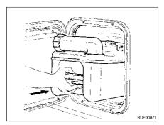
Fig. 259 Inserting the Thetford cassette
