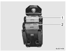
Fig. 173 Fuses for fuel cell
