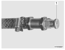
Fig. 282 Bleeding valve of hot-water heater
