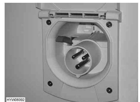
Fig. 90 230 V connection on vehicle
