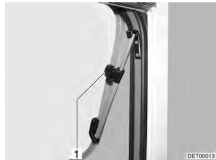
Fig. 55 Hinged window with rotary hinges, open
