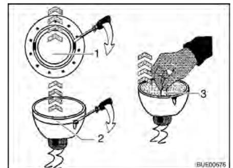
Fig. 254 Changing the halogen bulb
