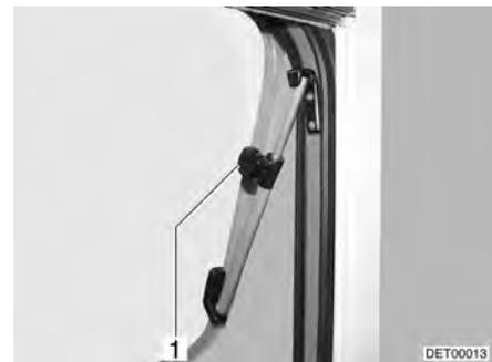
Fig. 79 Skylight with rotary hinges, open
