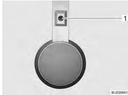
Fig. 46 Toilet compartment lighting, light switch directly on the lamp
