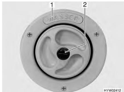
Fig. 201 Cap for the drinking water filler neck
