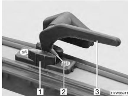
Fig. 61 Catch lever without safety knob in "continuous ventilation" position
