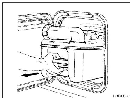
Fig. 235 Removing the Thetford cassette
