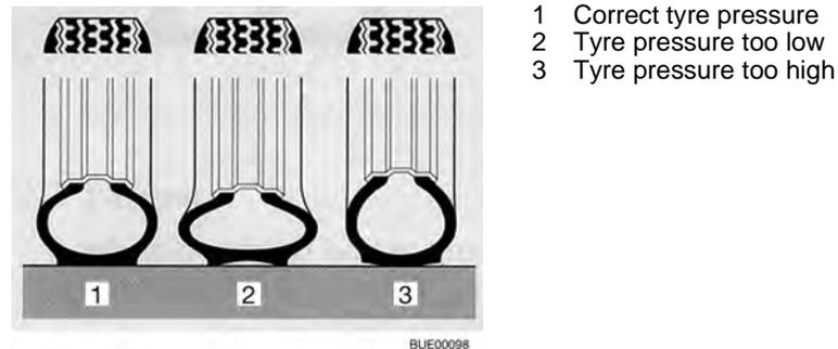
Fig. 266 Contact surface of the tyre
