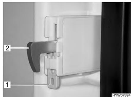
Fig. 198 Lock hook fixture
