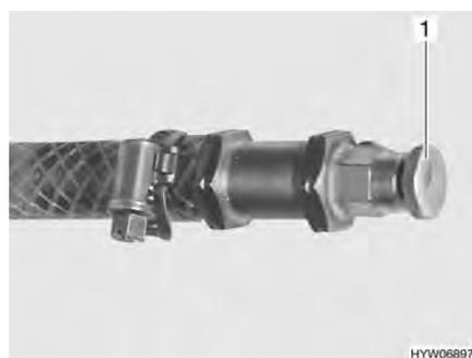
Fig. 248 Bleeding valve of hot-water heater
