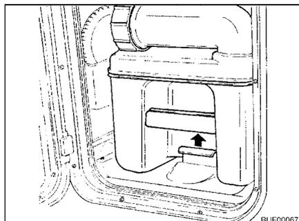
Fig. 210 Pulling the retaining clip
