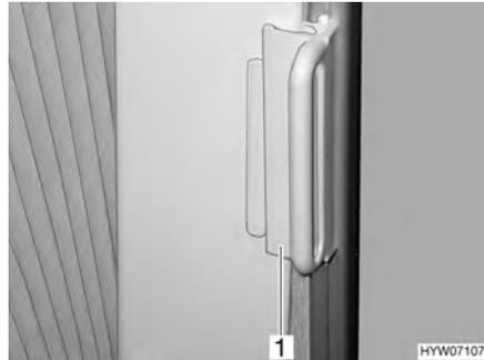
Fig. 23 Locking mechanism for Roman shade on driver's/front passenger's windows
