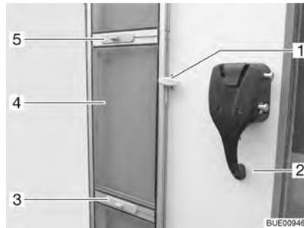
Fig. 32 Insect screen door, closed
