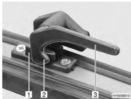
Fig. 59 Catch lever without safety knob in "closed" position
