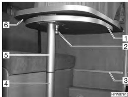
Fig. 82 Suspension table with separable support leg
