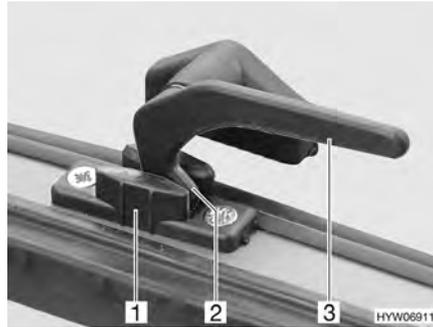
Fig. 56 Catch lever in the "continuous ventilation" position
