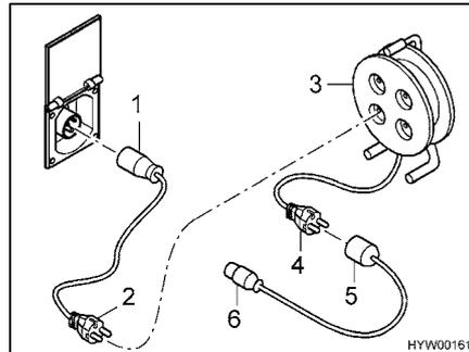
Fig. 136 Connection possibilities 230 V connection
