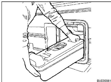
Fig. 211 Removing the Thetford cassette
