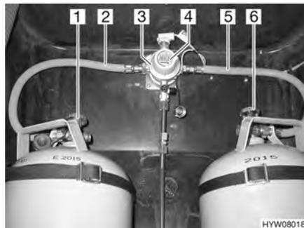
Fig. 129 DuoControl switching facility
