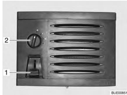
Fig. 165 Operating controls for auxiliary heat exchanger
