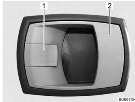
Fig. 30 Door lock of conversion door, inside
