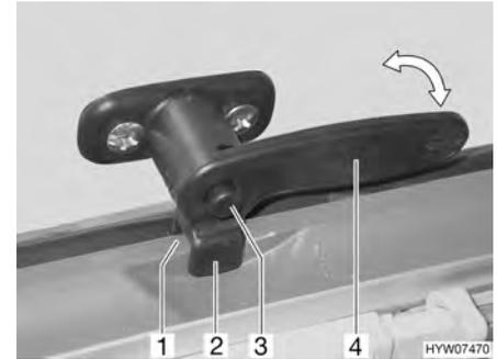
Fig. 62 Catch lever with safety knob in "continuous ventilation" position
