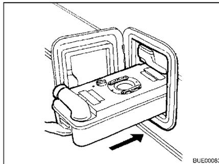
Fig. 214 Inserting the Thetford cassette
