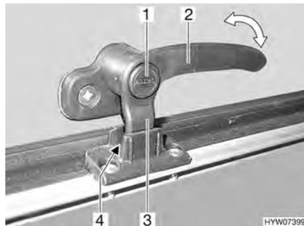
Fig. 65 Catch lever in the "continuous ventilation" position
