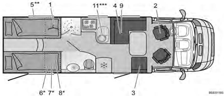
Fig. 283 Ground plan T 728 Nexxo
