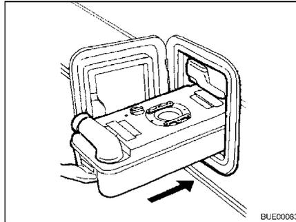
Fig. 230 Inserting the Thetford cassette
