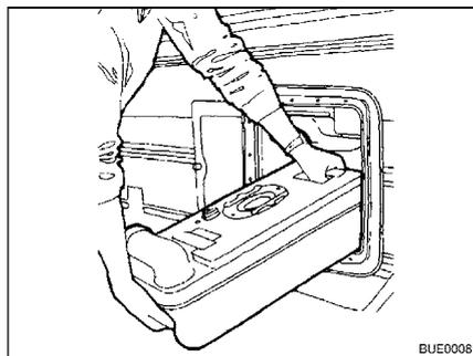
Fig. 227 Removing the Thetford cassette
