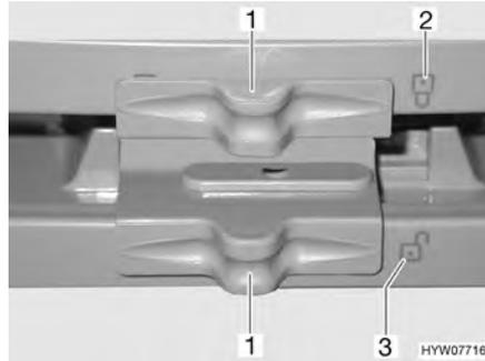
Fig. 195 Locking of the refrigerator door/freezer compartment door (Dometic 7 series with separate freezer compartment)
