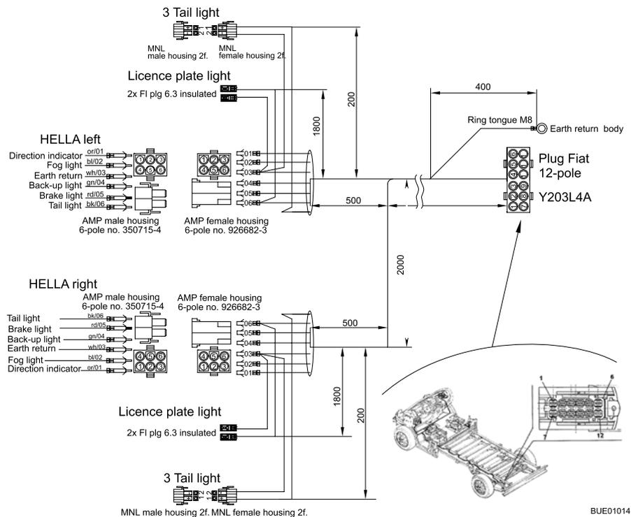
Fig. 153 Circuit diagram, exterior
