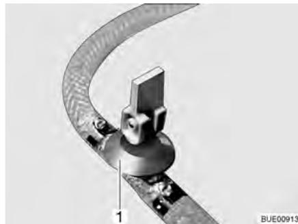
Fig. 208 Drain cock (with rocking lever)
