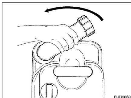
Fig. 212 Turning drainage neck
