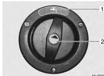
Fig. 202 Cap for the drinking water filler neck (alternative)
