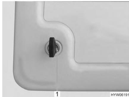
Fig. 37 Push-button lock service flap
