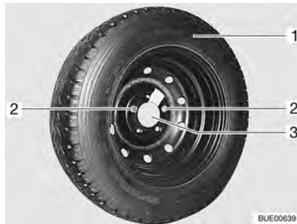
Fig. 265 Spare wheel support in the rear garage
