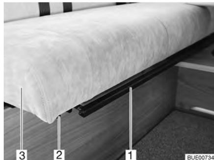
Fig. 20 Backrest adjustment mechanism for bench
