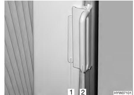
Fig. 72 Roman shades for driver's window and front passenger's window
