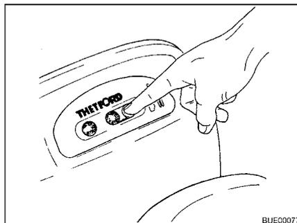
Fig. 221 Closing the sliding trap
