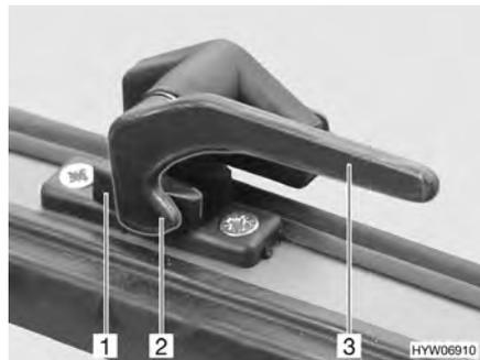
Fig. 54 Catch lever in "closed" position
