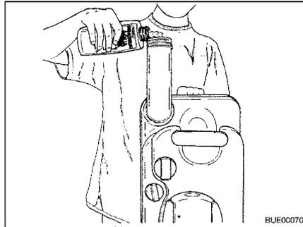
Fig. 213 Filling with sanitary liquid
