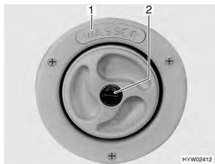
Fig. 39 Cap for the drinking water filler neck
