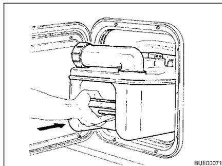
Fig. 238 Inserting the Thetford cassette
