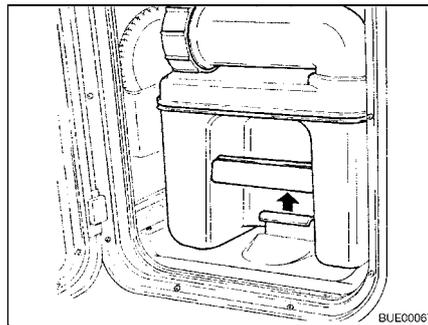
Fig. 226 Pulling the retaining clip
