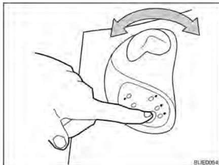
Fig. 234 Operating the flush
