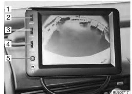
Fig. 18 LCD monitor for reversing camera
