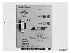
Fig. 144 Solar charge regulator fuse
