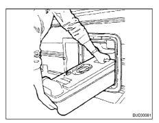
Fig. 227 Removing the Thetford cassette
