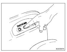
Fig. 220 Opening the sliding trap
