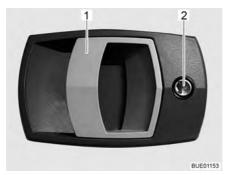
Fig. 29 Door lock of conversion door, outside
