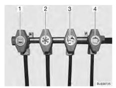
Fig. 125 Symbols for the gas isolator taps
