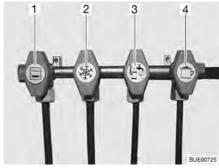
Fig. 154 Symbols for the gas isolator taps
