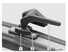
Fig. 80 Catch lever in the "continuous ventilation" position
