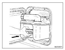
Fig. 238 Inserting the Thetford cassette
