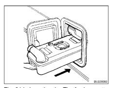
Fig. 214 Inserting the Thetford cassette
