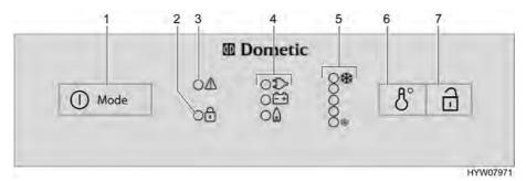
Fig. 191 Operating controls for the refrigerator (Dometic 8 series with MES)
