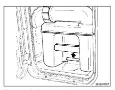
Fig. 226 Pulling the retaining clip
