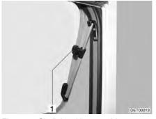
Fig. 79 Skylight with rotary hinges, open
