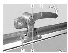
Fig. 65 Catch lever in the "continuous ventilation" position
