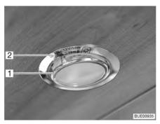
Fig. 255 Recessed halogen light (flat)
