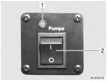
Fig. 164 Operating switch for auxiliary circulating pump
