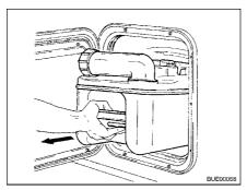
Fig. 222 Removing the Thetford cassette
