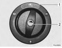
Fig. 40 Cap for the drinking water filler neck (alternative)
