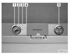
Fig. 189 Operating controls for the refrigerator (Dometic 7 series)
