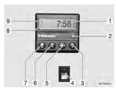
Fig. 168 Operating unit for independent vehicle heater
