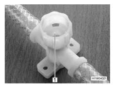
Fig. 206 Drain cock (with rocking lever)
