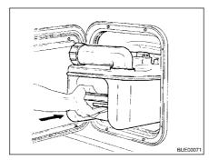
Fig. 225 Inserting the Thetford cassette
