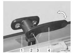
Fig. 60 Catch lever with safety knob in "closed" position
