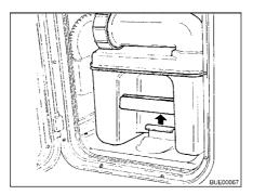
Fig. 210 Pulling the retaining clip
