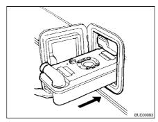
Fig. 230 Inserting the Thetford cassette
