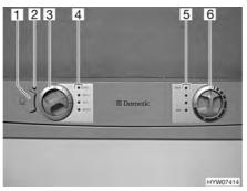
Fig. 190 Operating controls for the refrigerator (Dometic 7 series with AES and FH)
