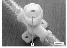
Fig. 208 Drain cock (with rocking lever)
