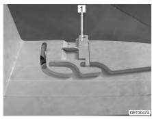
Fig. 76 Ventilation position locking mechanism
