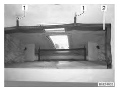
Fig. 101 Pull-down bed complete with applied safety net
