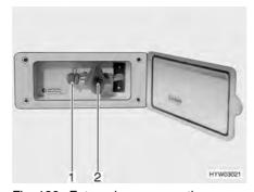
Fig. 126 External gas connection, gas isolator tap closed
