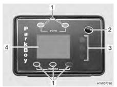
Fig. 16 Parking distance control operating unit
