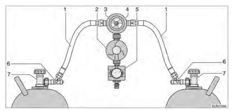
Fig. 127 Crash-Protection-Unit switching facility
