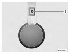
Fig. 46 Toilet compartment lighting, light switch directly on the lamp
