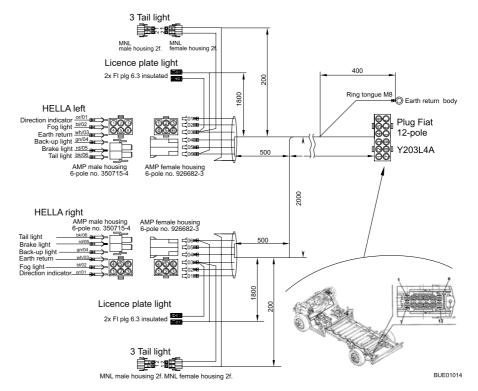
Fig. 153 Circuit diagram, exterior
