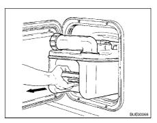
Fig. 235 Removing the Thetford cassette
