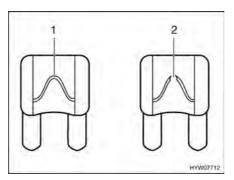
1 Unbroken fuse element 2 Broken fuse element
