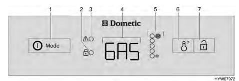
Fig. 192 Operating controls for the refrigerator (Dometic 8 series with AES)
