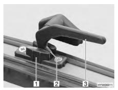
Fig. 61 Catch lever without safety knob in "continuous ventilation" position
