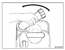
Fig. 228 Turning drainage neck
