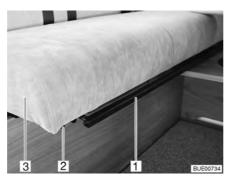
Fig. 20 Backrest adjustment mechanism for bench
