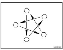
Fig. 261 Tighten the wheel nuts or wheel bolts cross-wise
