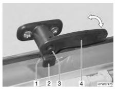
Fig. 62 Catch lever with safety knob in "continuous ventilation" position
