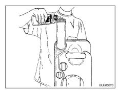
Fig. 213 Filling with sanitary liquid
