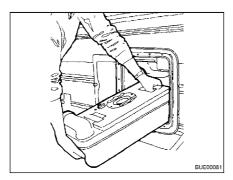
Fig. 211 Removing the Thetford cassette
