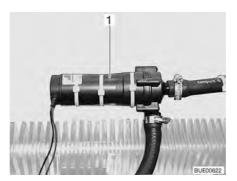
Fig. 163 Auxiliary circulating pump
