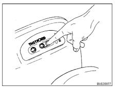
Fig. 221 Closing the sliding trap
