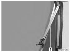
Fig. 58 Hinged window with automatic hinges
