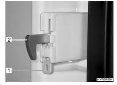
Fig. 198 Lock hook fixture
