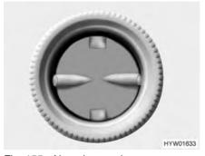
Fig. 155 Air outlet nozzle
