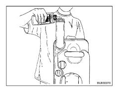
Fig. 241 Turning drainage neck
