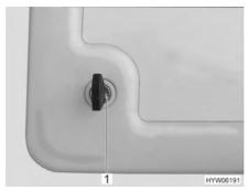
Fig. 37 Push-button lock service flap
