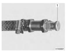
Fig. 248 Bleeding valve of hot-water heater
