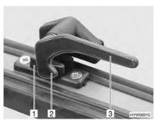
Fig. 59 Catch lever without safety knob in "closed" position
