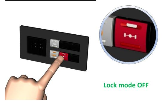
press the control switch again to unlock the rear differential. Audible and light signals
