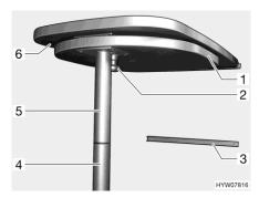
Fig. 25 Suspension table with separable support leg
