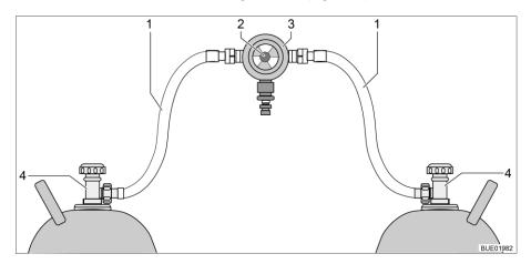
Fig. 63 Gas bottle switching facility
