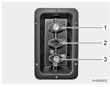
Fig. 77 Gas isolator taps position (example)
