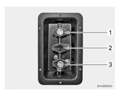
Fig. 68 Gas isolator taps position (example)
