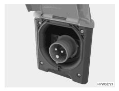
Fig. 72 230 V connection on the vehicle (CEE socket outlet)
