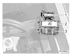
Fig. 74 Fuses on the starter battery
