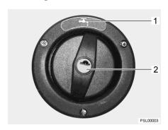
Fig. 93 Cap for the drinking water filler neck
