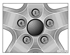
Fig. 113 Tightening the wheel nuts or wheel bolts cross-wise
