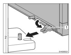
Fig. 91 Refrigerator door locking mechanism
