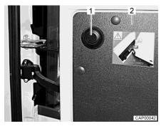
Fig. 10 Push button to release the limitation
