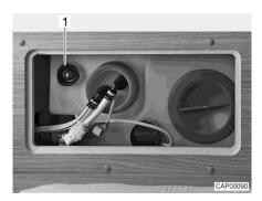
Fig. 97 Water tank with rotary han-
