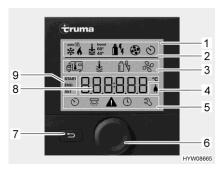
Fig. 80 Operating unit with displays
