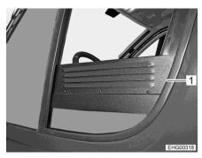
Fig. 53 Forced ventilation grille (side window open)
