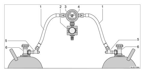
Fig. 5 Gas regulator with CPU and hose break guard
