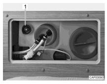
Fig. 96 Water tank with rotary handle
