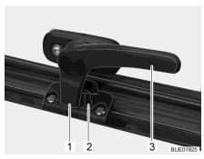
Fig. 11 Catch lever in "closed" position
