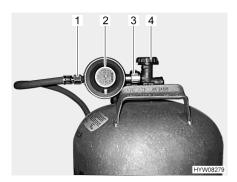
Fig. 67 Gas bottle connection
