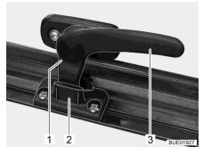
Fig. 13 Catch lever in "continuous ventilation" position
