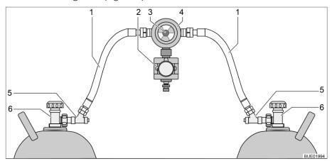
Fig. 64 Gas bottle switching facility with CPU
