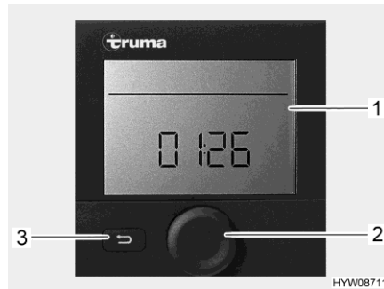
Fig. 72 Operating unit (hot-air heater and boiler)
