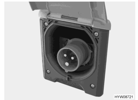
Fig. 65 230 V connection on the vehicle (CEE socket outlet)
