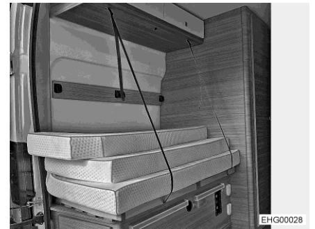
Fig. 39 Transport position (removable bed base)
