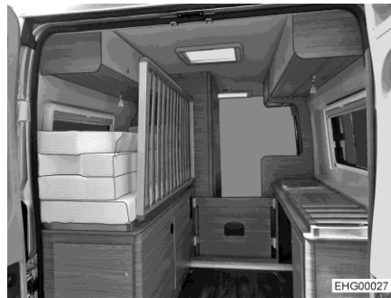
Fig. 38 Transport position (folding bed base)
