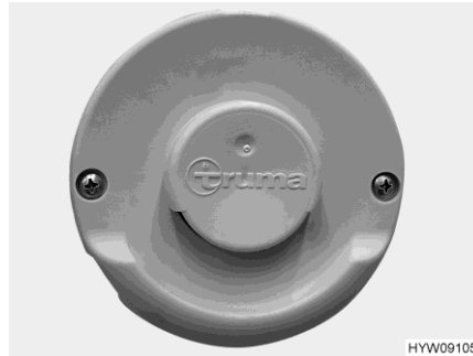
Fig. 77 Wall flue (hot-air heater)
