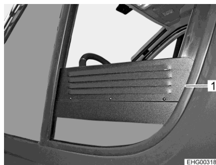
Fig. 46 Forced ventilation grille (side window open)
