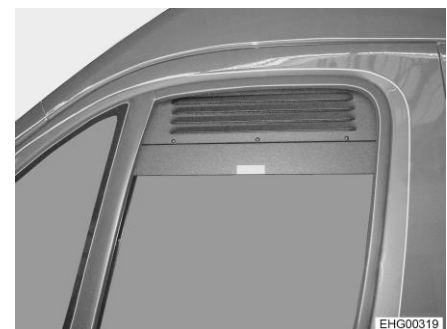
Fig. 47 Forced ventilation grille (side window closed)
