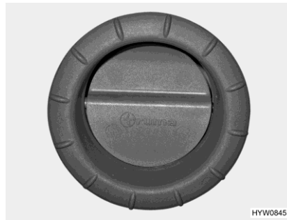
Fig. 71 Air outlet nozzle (hot-air heater)
