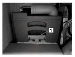
Fig. 145: Waste holding tank in the disposal shaft
