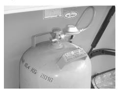
Fig. 103: Gas bottle with pressure reducing valve
