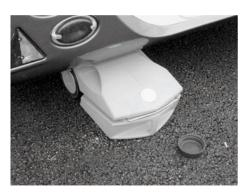
Fig. 101: Wheeled waste water tank
