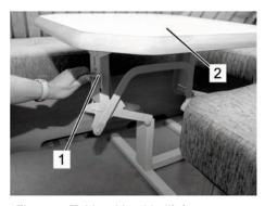
Fig. 134: Table with table lift frame
