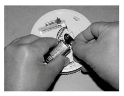
Fig. 111: Replacing the block battery
