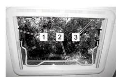
Fig. 121: Operating the Heki 2 lift skylight
