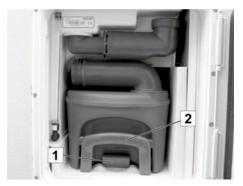
Fig. 142: Waste holding tank in the disposal shaft
