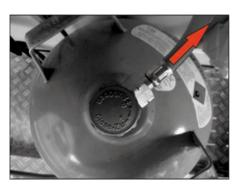
Fig. 78: Gas bottle alignment
