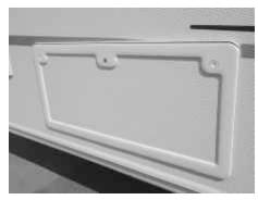
Fig. 29: Service compartment on the outside of the caravan
