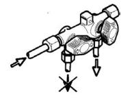
Fig. 82: Shut-off and release position
