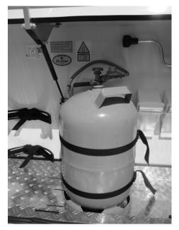
Fig. 76: Open gas locker
