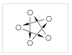
Fig. 156: Always tighten tyre nuts and bolts crosswise
