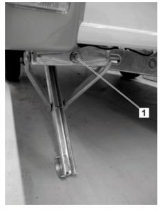
Fig. 15: Hexagonal bolt (1) for socket wrench
