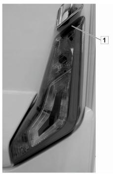
Fig. 167: Undoing the hybrid light
