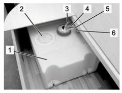
Fig. 88: Fresh water tank, example
