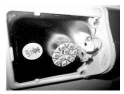
Fig. 161: Replacing LEDs
