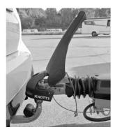
Fig. 13: Tow-ball coupling opened, stabilisation deactivated
