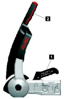
Fig. 5: Tow-ball coupling open
