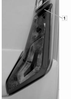
Reach into the hole on the rear side of the housing. Rotate 2. bulb holder (2) (bayonet fitting) and pull out. The brake lamp is shown here as an example.
