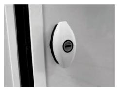
Fig. 30: Service compartment lock
