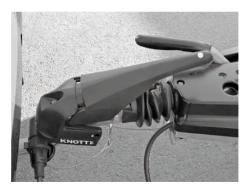
Fig. 10: Tow-ball coupling closed, stabilisation activated
