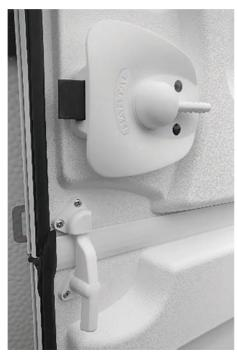
Fig. 27: Closed but unsecured door lock
