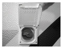
Fig. 87: Fresh water intake port
