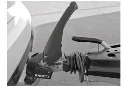
Fig. 9: Tow-ball coupling closed, stabilisation deactivated
