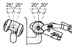
Fig. 4: Maximum swivel range of the ball coupling on the coupling ball of the towing vehicle.
