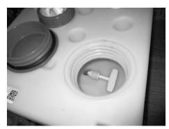
Fig. 91: Drain plug in the fresh water tank
