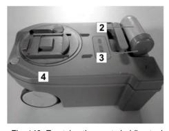
Fig. 146: Emptying the waste holding tank
