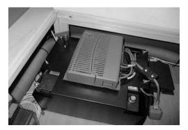
Fig. 66: Battery cover with control module for mover (optional)
