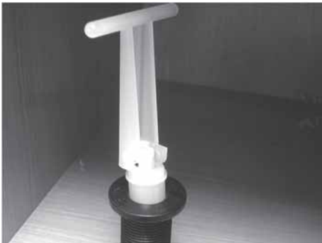
Fig. 107: Drain plug in fresh water tank, open (rocker lever straight)
