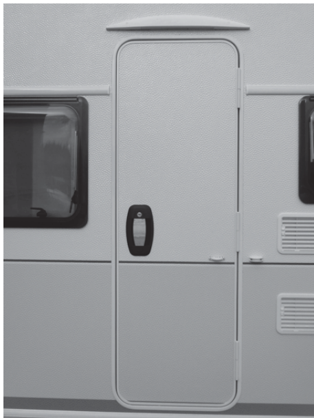
Fig. 11: Entrance door without window (example)
