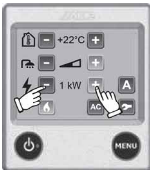
Fig. 170: Heating with electricity
