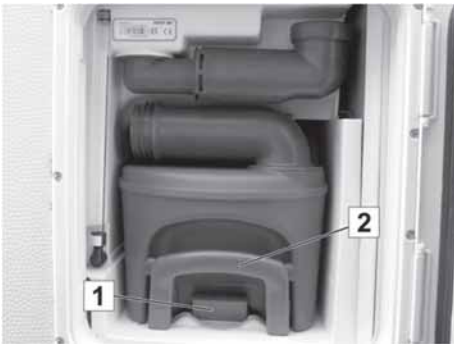
Fig. 200: Waste holding tank in the disposal shaft
