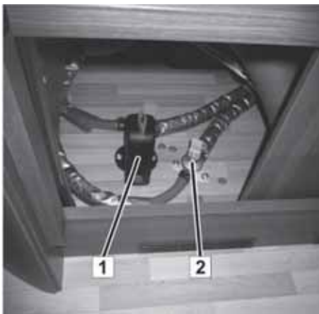
Fig. 108: TRUMA combination heater drain valves
