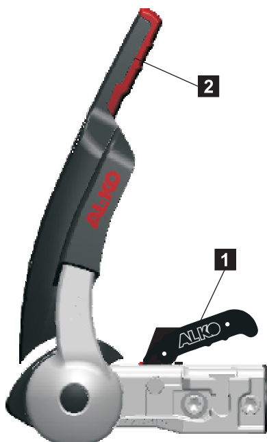
Fig. 8: "AL-KO" safety coupling
