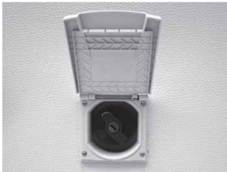
Fig. 92: Fresh water intake port
