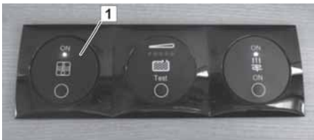
Fig. 100: On-Off switch of the water heating system
