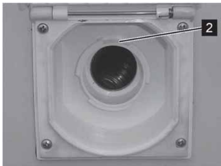
Fig. 106: Fresh water intake port, open
