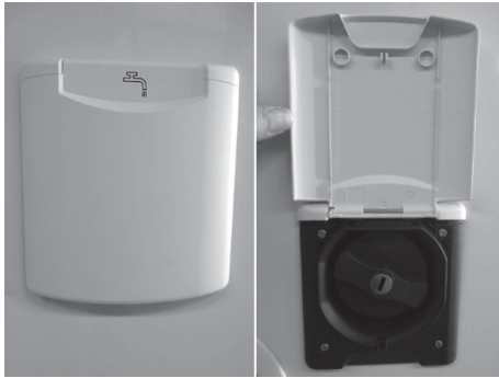
Fig. 104: Fresh water intake port
