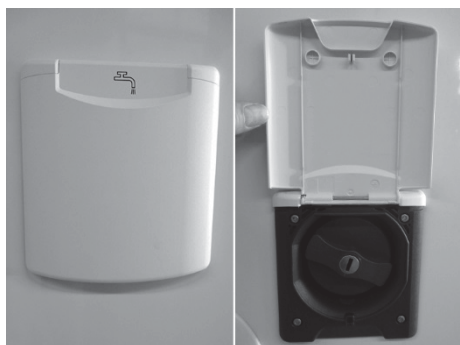
Fig. 21: Fresh water intake port
