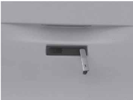
Fig. 73: Gas bottle locker lock unlocked
