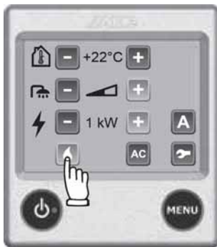
Fig. 169: Heating with gas
