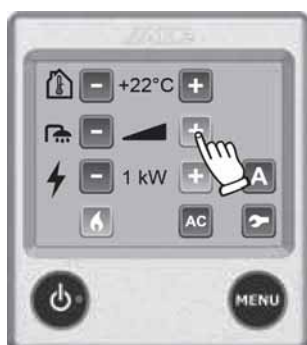
Fig. 168: More hot water
