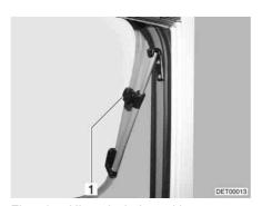
Fig. 59 Hinged window with rotary hinges
