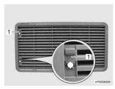
Fig. 162 Refrigerator ventilation grill (with sliding trap)
