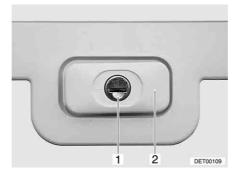
Fig. 36 Flap lock, rectangular, closed
