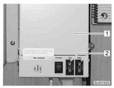
Fig. 125 Heater regulation for waste water pipes
