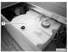
Fig. 194 Cleaning opening water tank
