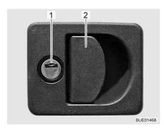
Fig. 35 Flap lock with recessed handle
