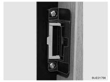
Fig. 176 Locking device in ventilation position
