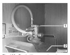
Fig. 108 Gas bottle compartment
