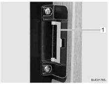
Fig. 175 Locking device in normal position
