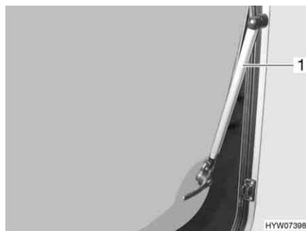
Fig. 64 Hinged window with automatic hinges
