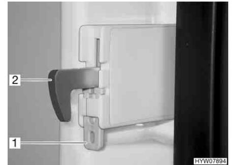
Fig. 174 Lock hook fixture
