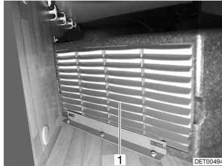
Fig. 200 Air conditioning unit (Truma)
