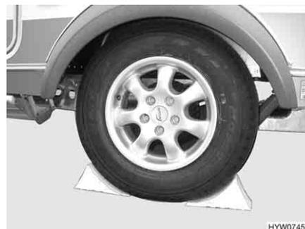
Fig. 224 Securing vehicle
