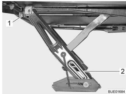
Fig. 24 Corner steady with footplate (cranked down)
