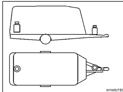
Fig. 8 Incorrect weight distribution
