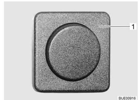
Fig. 43 Interior light, light switch separate from the lamp
