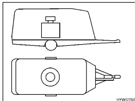
Fig. 9 Correct weight distribution
