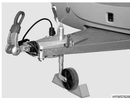
Fig. 232 Securing support wheel
