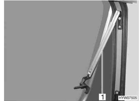
Fig. 56 Hinged window with automatic hinges, open
