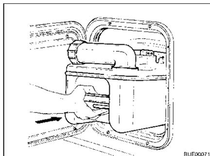
Fig. 201 Inserting the Thetford cassette
