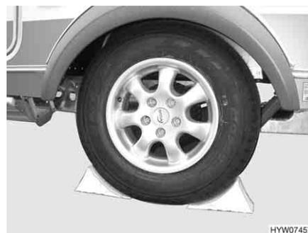
Fig. 233 Securing vehicle
