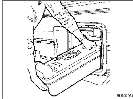
Fig. 171 Removing the Thetford cassette
