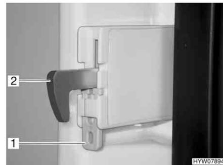
Fig. 156 Lock hook fixture
