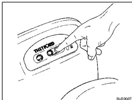
Fig. 181 Closing the sliding trap
