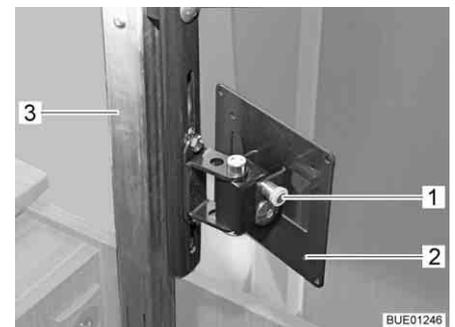
Fig. 51 Lifting mechanism
