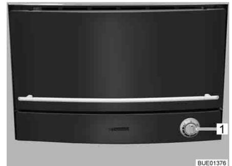
Fig. 146 Gas oven (Dometic)
