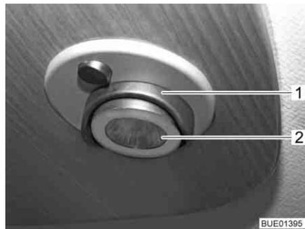
Fig. 217 Recessed halogen light
