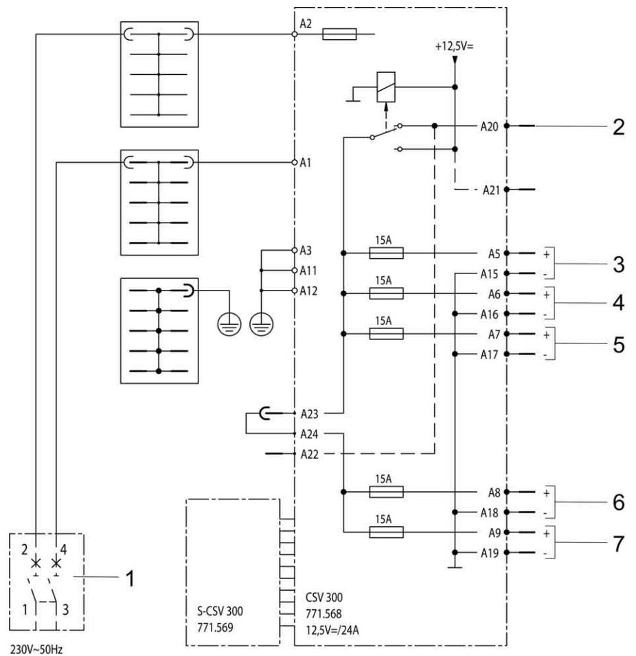
Fig. 119 Circuit diagram, interior (CSV 300)
