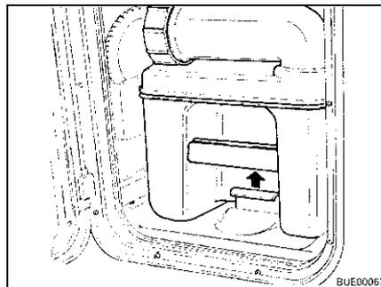
Fig. 170 Pulling the retaining clip
