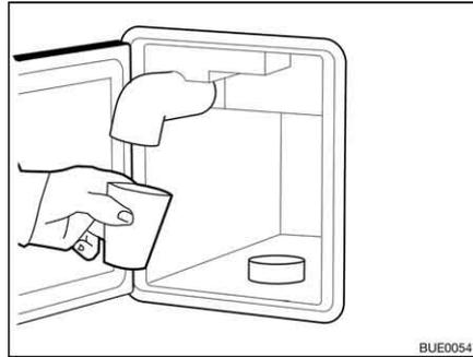
Fig. 203 Emptying the fresh water filler neck
