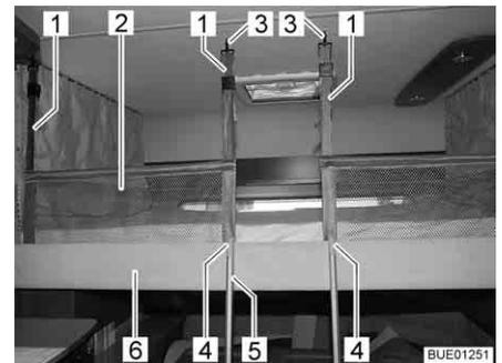
Fig. 79 Pull-down bed complete with applied safety net
