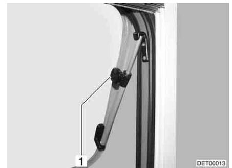
Fig. 53 Hinged window with rotary hinges, open
