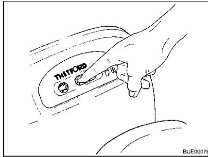
Fig. 180 Opening the sliding trap
