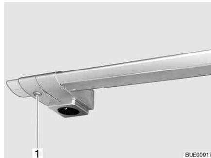
Fig. 42 Interior light, switch mounted directly on the lamp
