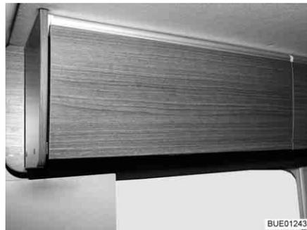
Fig. 39 Furniture flaps with pressurised release (example)
