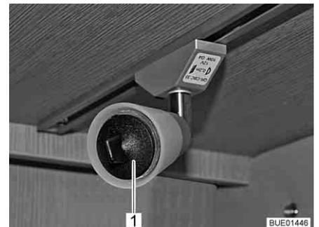
Fig. 225 Suction cup for replacing the lamp
