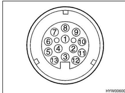
Fig. 115 Contact diagram of the thirteen-pin plug
