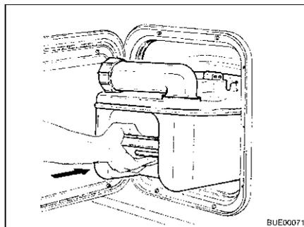
Fig. 185 Inserting the Thetford cassette
