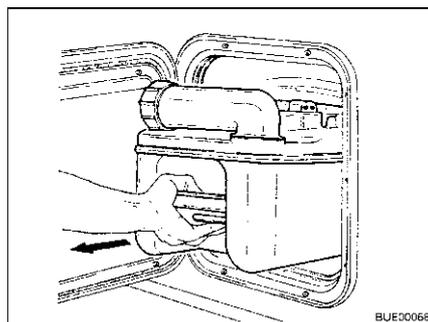
Fig. 182 Removing the Thetford cassette
