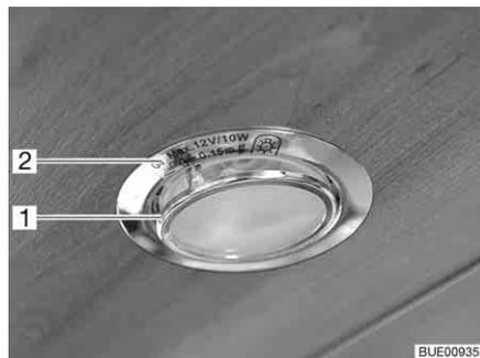
Fig. 218 Recessed halogen light (flat)
