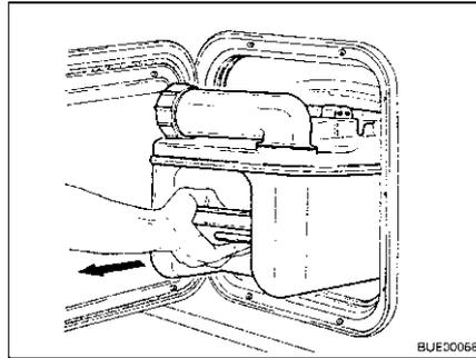
Fig. 198 Removing the Thetford cassette
