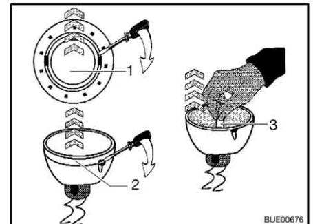
Fig. 216 Changing the halogen bulb
