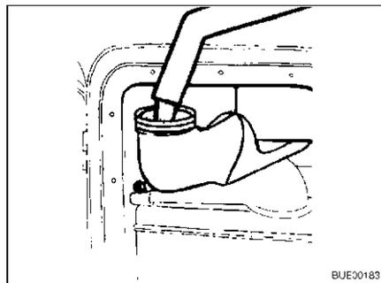
Fig. 187 Filling with fresh water
