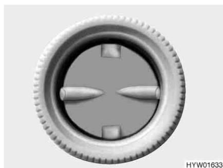
Fig. 122 Air outlet nozzle
