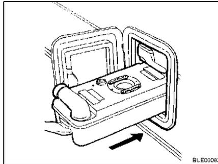
Fig. 174 Inserting the Thetford cassette
