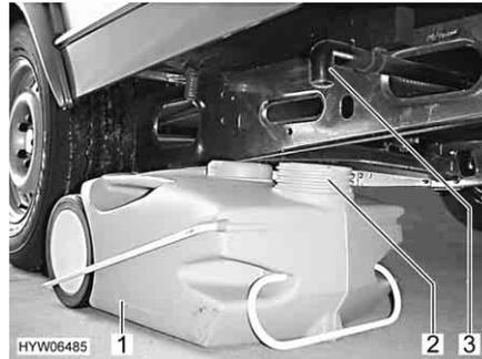
Fig. 22 Waste water tank, mobile
