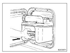
Fig. 192 Inserting the Thetford cassette
