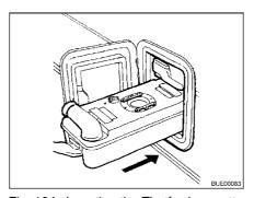
Fig. 184 Inserting the Thetford cassette
