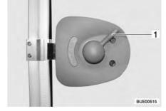
Fig. 24 Door lock of conversion door, inside, open
