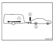
Fig. 9 Caravan load, nose weight and axle load
