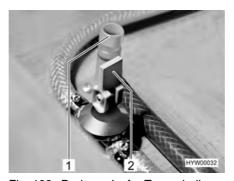
Fig. 132 Drain cocks for Truma boiler
