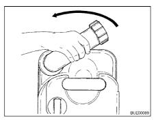
Fig. 163 Turning drainage neck
