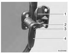
Fig. 29 Window in the conversion door, catch lever closed
