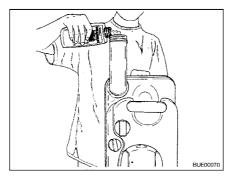
Fig. 183 Filling with sanitary liquid
