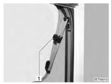
Fig. 52 Catch lever in "closed" position
