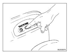
Fig. 171 Opening the sliding trap
