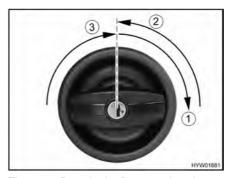
Fig. 22 Door lock of conversion door, outside, opening
