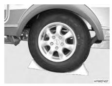
Fig. 218 Securing support wheel
