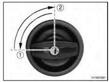
Fig. 23 Door lock of conversion door, outside, locking
