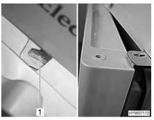
Fig. 145 Refrigerator door in ventilation position (Dometic 7 series)
