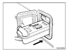
Fig. 165 Inserting the Thetford cassette
