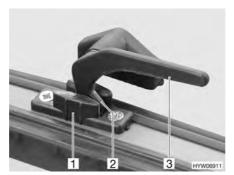
Fig. 54 Catch lever in the "continuous ventilation" position
