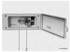
Fig. 97 External gas connection, gas isolator tap closed
