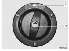
Fig. 39 Cap for the drinking water filler neck (alternative)
