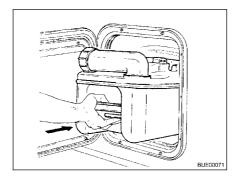
Fig. 176 Inserting the Thetford cassette
