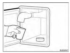
Fig. 194 Emptying the fresh water filler neck
