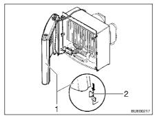
Fig. 119 Heater cover, retaining clips
