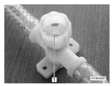
Fig. 159 Drain cock (with rocking lever)
