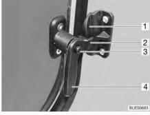
Fig. 30 Window in the conversion door in the "continuous ventilation" position
