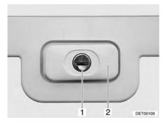
Fig. 35 Flap lock, rectangular, closed
