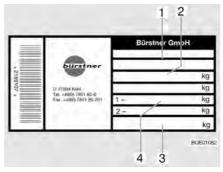
Fig. 215 Vehicle identification plate
