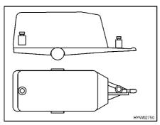
Fig. 7 Incorrect weight distribution
