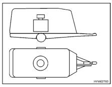
Fig. 8 Correct weight distribution
