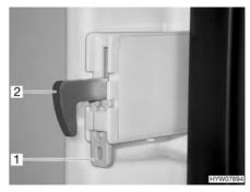
Fig. 149 Lock hook fixture
