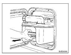
Fig. 173 Removing the Thetford cassette
