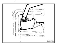
Fig. 178 Filling with fresh water
