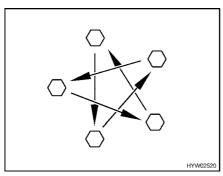
Fig. 216 Tighten the wheel nuts or wheel bolts cross-wise
