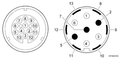
Fig. 108 Contact diagram of the thirteen-pin plug
