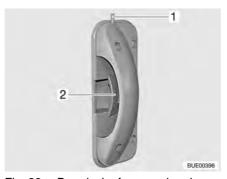
Fig. 28 Door lock of conversion door, inside
