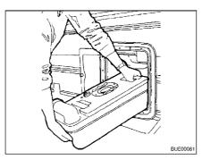
Fig. 181 Removing the Thetford cassette
