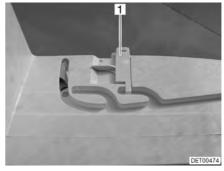
Fig. 62 Ventilation position locking mechanism
