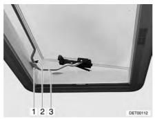
Fig. 65 Heki skylight in ventilation position 2
