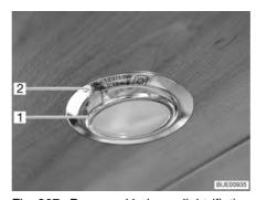
Fig. 207 Recessed halogen light (flat)
