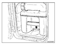
Fig. 161 Pulling the retaining clip
