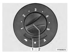
Fig. 120 Operating switch for circulation fan
