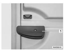
Fig. 26 Catch lever on the lower part of the door
