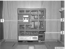
Fig. 101 Power supply unit CSV 300
