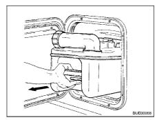
Fig. 189 Removing the Thetford cassette
