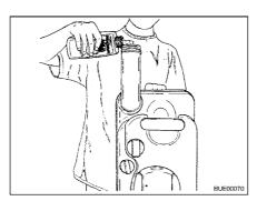
Fig. 164 Filling with sanitary liquid
