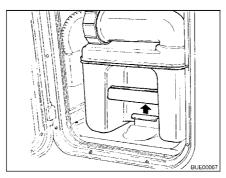
Fig. 180 Pulling the retaining clip
