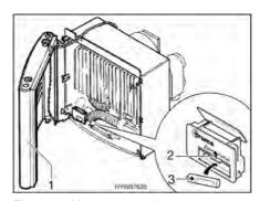
Fig. 117 Removing heater cover
