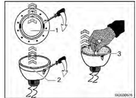
Fig. 206 Changing the halogen bulb
