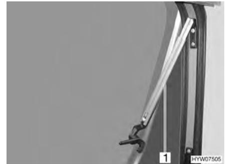
Fig. 56 Hinged window with automatic hinges, open
