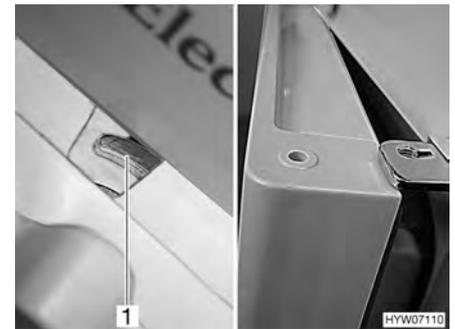
Fig. 145 Refrigerator door in ventilation position (Dometic 7 series)
