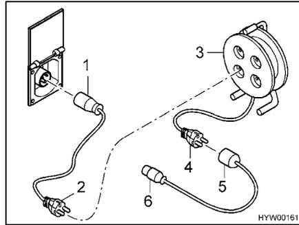
Fig. 102 Connection possibilities 230 V connection
