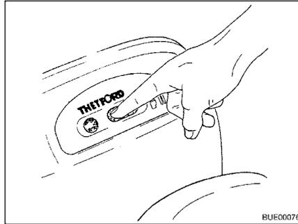
Fig. 171 Opening the sliding trap
