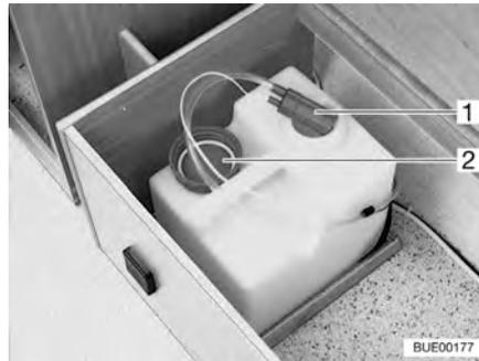
Fig. 152 Water tank 16 l
