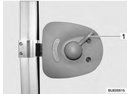
Fig. 25 Door lock of conversion door, inside, locked
