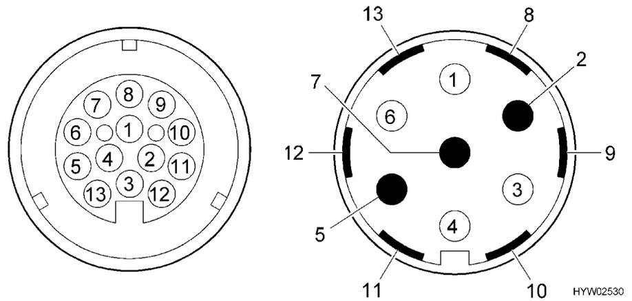
Fig. 108 Contact diagram of the thirteen-pin plug
