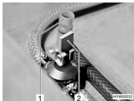
Fig. 132 Drain cocks for Truma boiler
