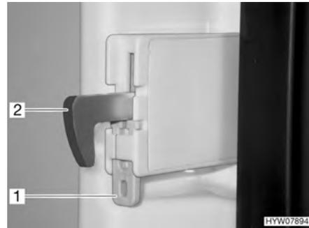
Fig. 149 Lock hook fixture
