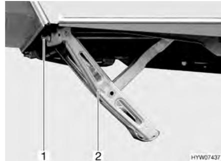
Fig. 19 Corner steady cranked down (variant 2)
