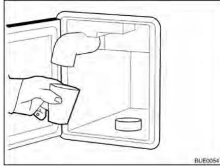
Fig. 194 Emptying the fresh water filler neck
