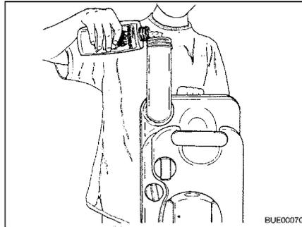
Fig. 183 Filling with sanitary liquid
