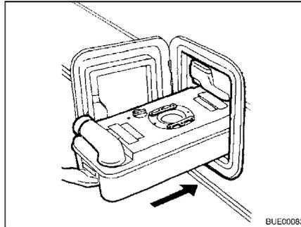
Fig. 165 Inserting the Thetford cassette
