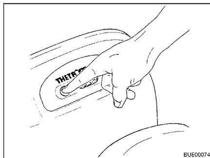
Fig. 170 Operating the flush
