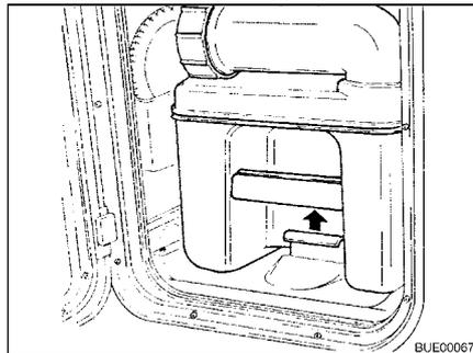
Fig. 180 Pulling the retaining clip
