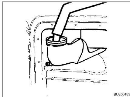
Fig. 178 Filling with fresh water
