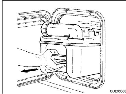
Fig. 189 Removing the Thetford cassette
