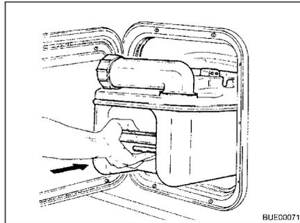
Fig. 192 Inserting the Thetford cassette
