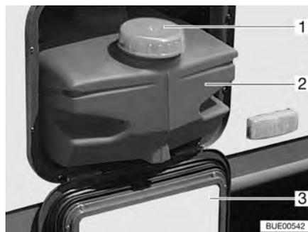
Fig. 153 Water tank 22 l
