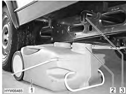
Fig. 21 Waste water tank, mobile
