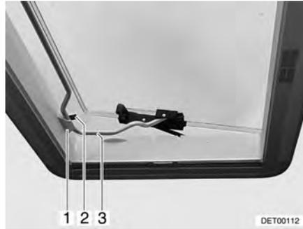
Fig. 65 Heki skylight in ventilation position 2
