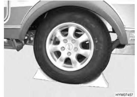
Fig. 219 Securing vehicle
