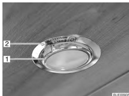
Fig. 207 Recessed halogen light (flat)
