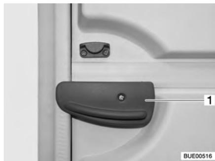
Fig. 26 Catch lever on the lower part of the door
