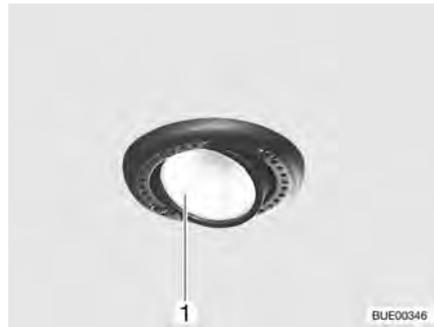
Fig. 205 Recessed halogen light
