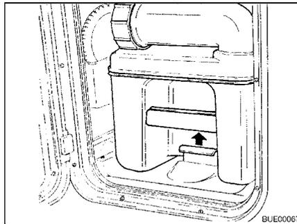
Fig. 161 Pulling the retaining clip
