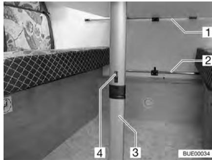
Fig. 67 Suspension table with folding leg
