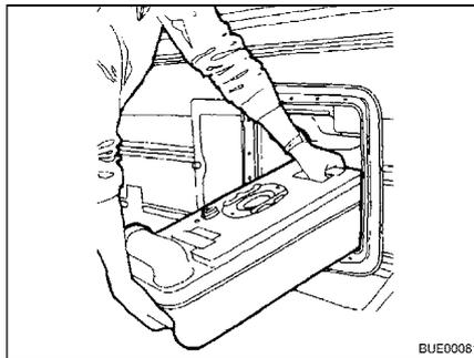
Fig. 162 Removing the Thetford cassette
