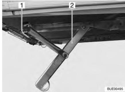
Fig. 18 Corner steady cranked down (variant 1)
