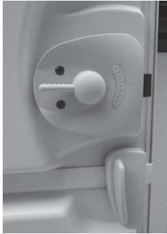
Fig. 20: Closed but unsecured door lock
