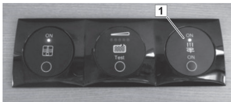
Fig. 127: On-Off switch of the floor heating system
