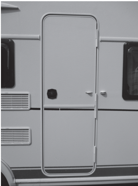
Fig. 17: Entrance door without window (example)
