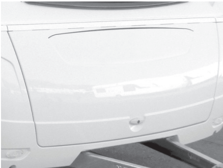
Fig. 73: Gas locker, closed
