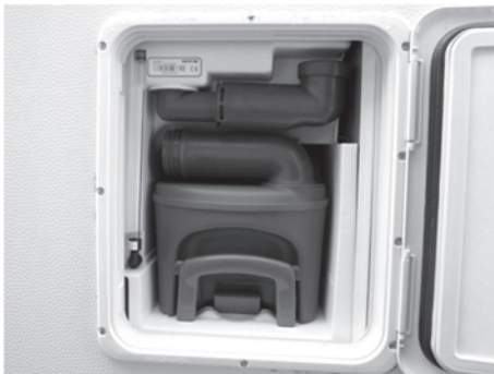
Fig. 47: Holding tank with flushing water intake port
