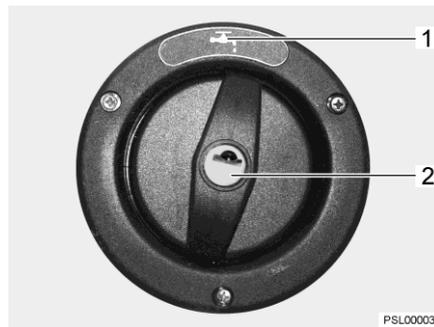
Fig. 169 Drinking water filler neck in the vehicle's side wall
