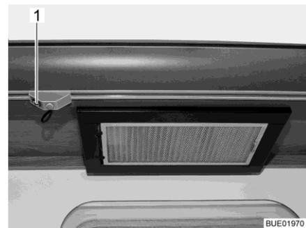
Fig. 160 Recirculating extractor hood
