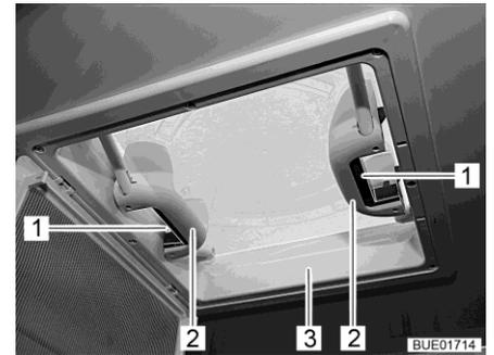
Fig. 85 Handles with snap latches
