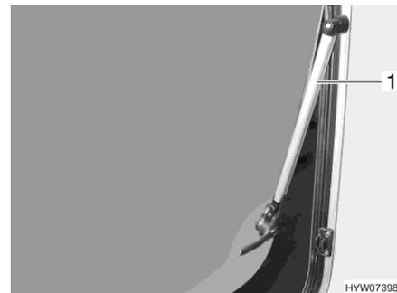
Fig. 72 Hinged window with automatic hinge
