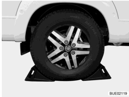
Fig. 211 Securing vehicle
