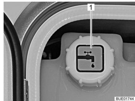
Fig. 170 Drinking water filler neck in service unit (alternative)
