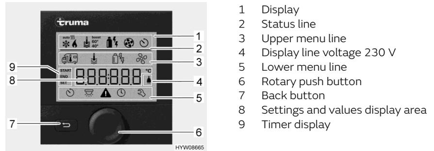
Fig. 142 Operating unit with displays
