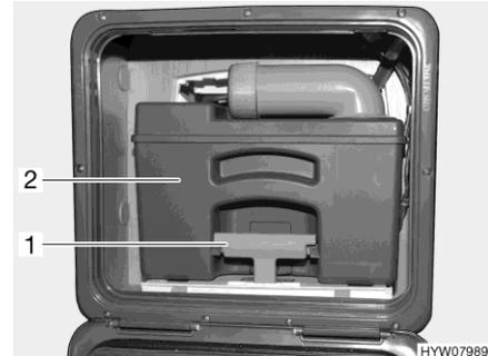
Fig. 188 Sewage tank (example)
