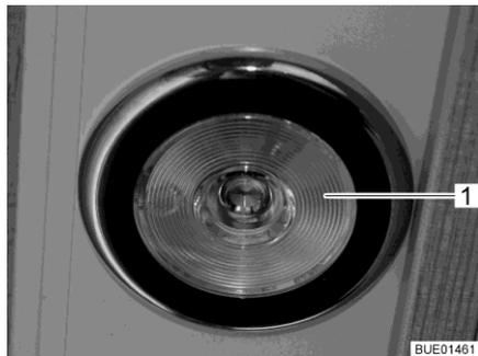
Fig. 61 Recessed light, light switch in the lamp
