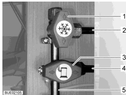
Fig. 110 Gas isolator taps position (example)
