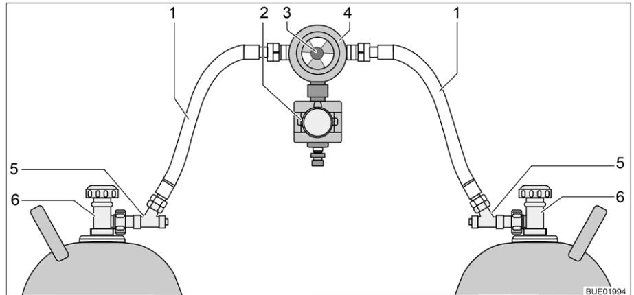
Fig. 16 Gas regulator with CPU and hose break guard
