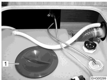
Fig. 196 Cleaning opening of the water tank
