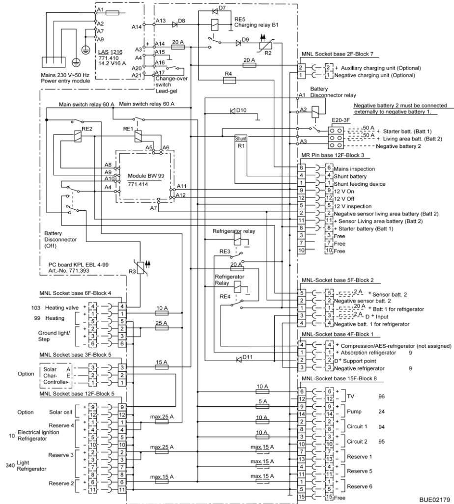
Fig. 136 Circuit diagram, interior (EBL 119)
