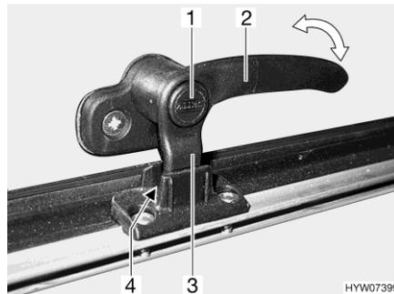
Fig. 73 Catch lever with safety knob in "continuous ventilation" position
