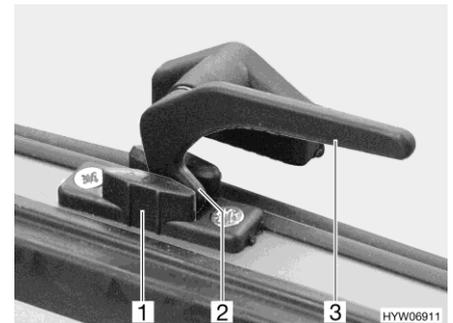
Fig. 74 Catch lever in "continuous ventilation" position
