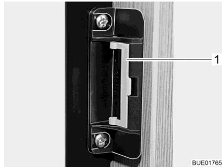
Fig. 166 Locking device in normal position
