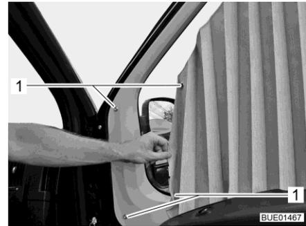
Fig. 80 Fixing of pleated shades
