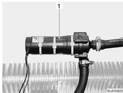
Fig. 149 Auxiliary circulating pump
