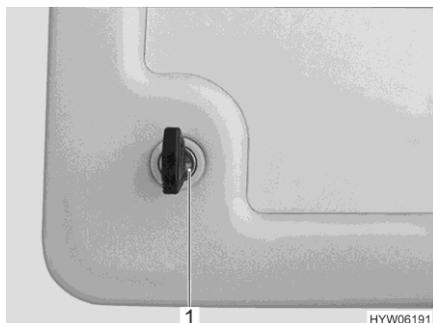
Fig. 46 Service flap push-button lock
