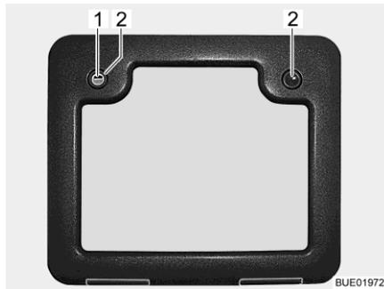
Fig. 193 Flap for the sewage tank
