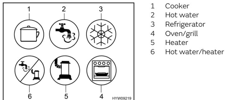
Fig. 139 Possible symbols for the gas isolator taps
