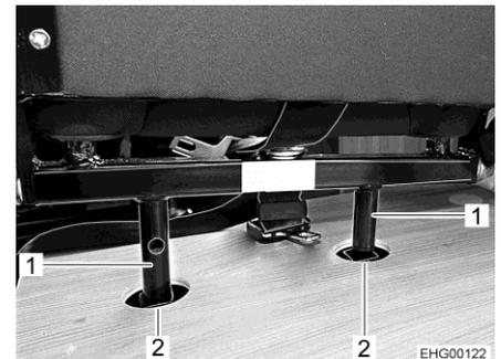
Fig. 23 Bars (inserted)
