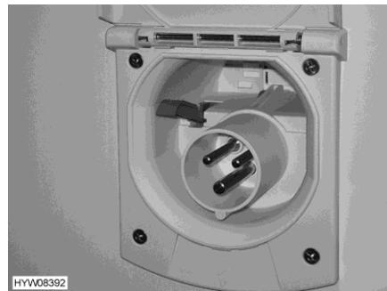
Fig. 124 230 V connection on the vehicle
