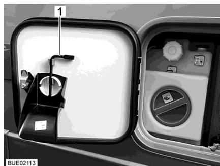
Fig. 184 Service flap with square spanner
