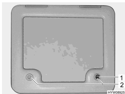
Fig. 99 Flap for the sewage tank
