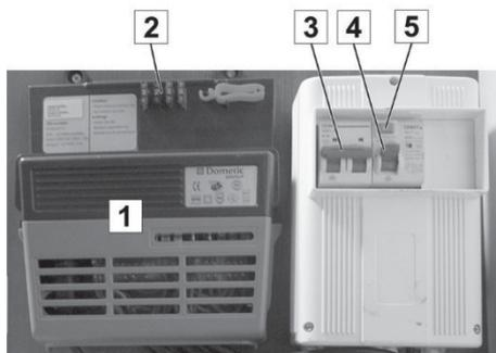
Fig. 61: Converter (power supply unit) (1) and cut-outs
