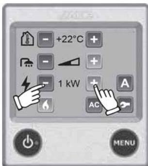
Fig. 167: Heating with electricity
