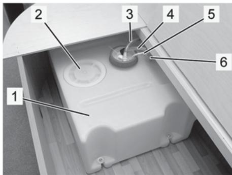
The fresh water tank is located in the living or sleeping area (shown in the Fig. under the bench seat of the sitting group as an example).
