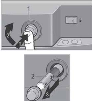
Fig. 209: Changing the batteries of the battery igniter (only if present)
