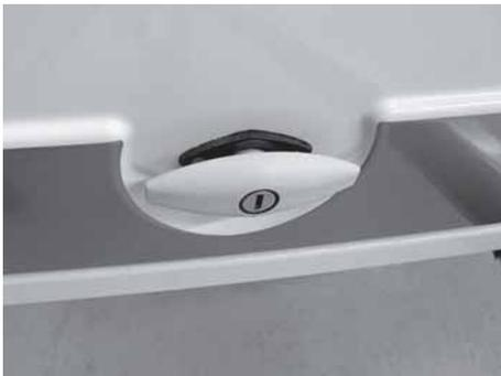
Fig. 20: Gas locker lock
