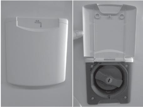
Fig. 102: Fresh water intake port
