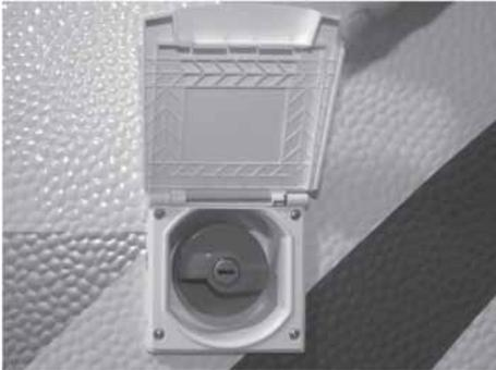
Fig. 91: Fresh water intake port
