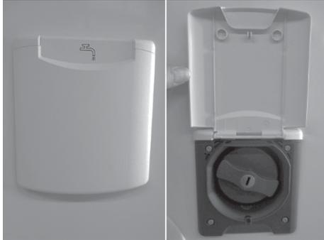
Fig. 90: Fresh water intake port
