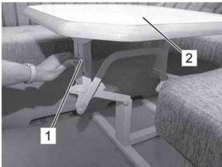
Fig. 178: Table with table lift frame
