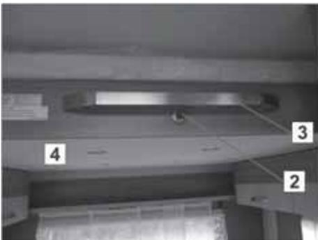
2. Press the knob (2) on the bed rail close to the pull-grip (3) so that the brake releases.
