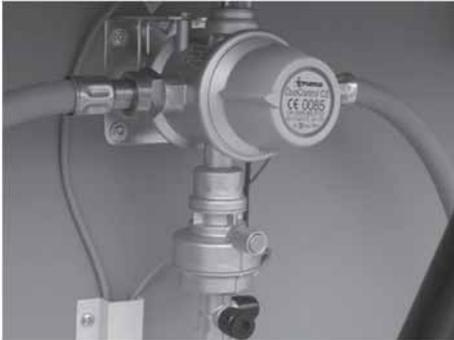
Fig. 76: Gas supply (with Eis-Ex and remote control)
