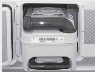
Fig. 45: Waste holding tank
