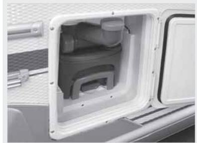
Fig. 46: Holding tank with flushing water intake port
