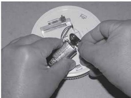
Fig. 217: Replacing the block battery
