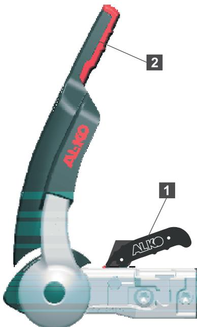
Fig. 5: Tow-ball coupling open
