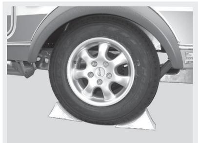
*Fig. 212: Securing the vehicle wheel*
