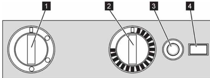
Fig. 208: Control elements on the refrigerator with manual ignition
