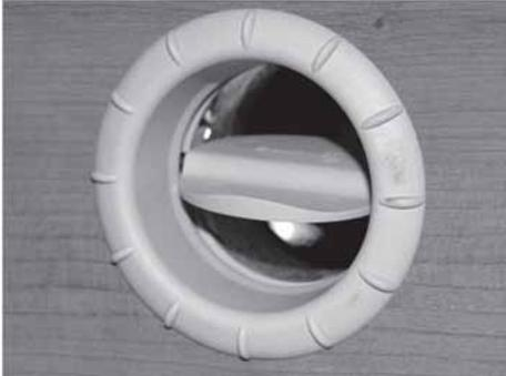
Fig. 133: Hot-air nozzle, open
