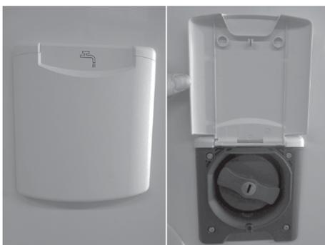
Fig. 21: Fresh water intake port
