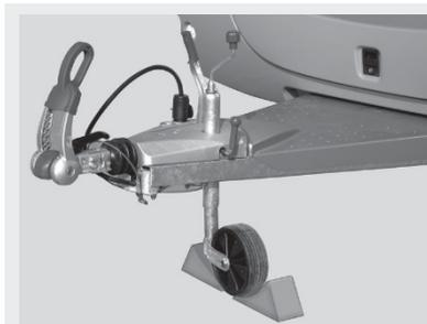
*Fig. 211: Securing the support wheel*
