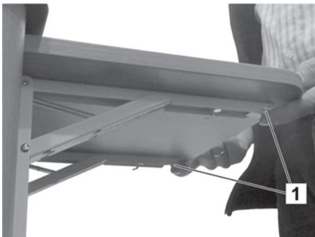
Fig. 182: Undoing the latching mechanism
