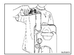
Fig. 255 Filling with sanitary liquid
