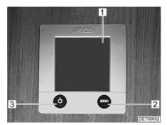
Fig. 202 Operating unit for hot-water heater
