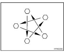
Fig. 304 Tighten the wheel nuts or wheel bolts cross-wise
