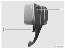
Fig. 42 Door lock of conversion door, inside, locked
