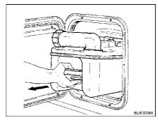
Fig. 277 Removing the Thetford cassette
