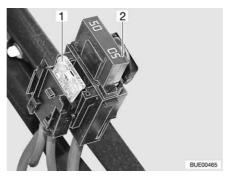
Fig. 181 Fuses on the starter battery
