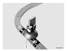
Fig. 248 Drain cock (with rocking lever)
