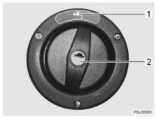
Fig. 50 Cap for the drinking water filler neck
