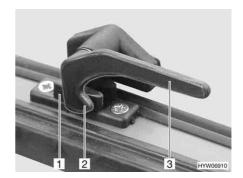
Fig. 69 Catch lever in "closed" position
