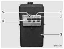
Fig. 189 230 V fuse box with safety cutout and FI-switch
