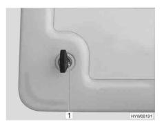
Fig. 48 Push-button lock service flap
