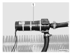
Fig. 208 Auxiliary circulating pump
