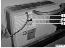
Fig. 174 Connector panel of the fuel cell
