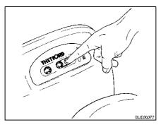
Fig. 263 Closing the sliding trap
