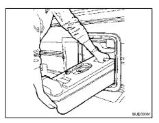
Fig. 269 Removing the Thetford cassette
