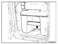
Fig. 252 Pulling the retaining clip
