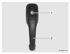
Fig. 41 Door lock of conversion door, outside
