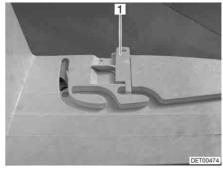
Fig. 87 Ventilation position locking mechanism
