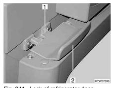
Fig. 241 Lock of refrigerator door, closed (Thetford)
