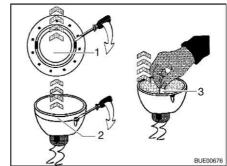
Fig. 294 Recessed halogen light (flat)
