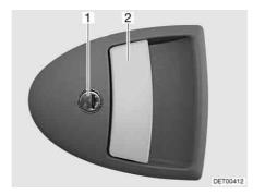
Fig. 43 Door lock of conversion door, outside
