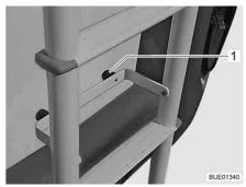
Fig. 3 Foldable ladder, ladder folded downwards
