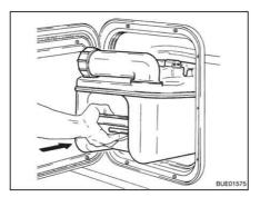
Fig. 256 Inserting the Thetford cassette
