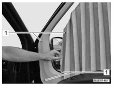
Fig. 81 Fixing of pleated shades
