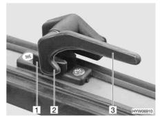
Fig. 74 Catch lever in "closed" position
