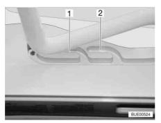
Fig. 86 Heki skylight in ventilation position
