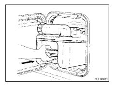
Fig. 267 Inserting the Thetford cassette
