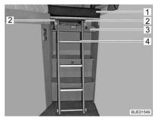
Fig. 119 Bed widening with access ladder
