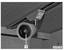
Fig. 300 Suction cup for replacing the lamp
