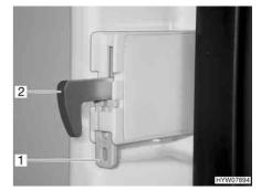
Fig. 238 Lock hook fixture
