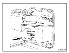
Fig. 280 Inserting the Thetford cassette
