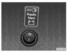
Fig. 169 Selector switch for operating behaviour
