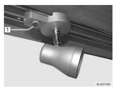
Fig. 58 Spotlight, switch mounted directly on the lamp
