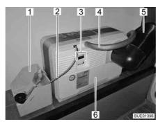
Fig. 173 Fuel cell with tank cartridge
