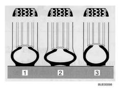
Fig. 310 Contact surface of the tyre
