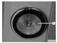
Fig. 60 Recessed light, light switch in the lamp
