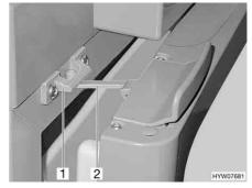
Fig. 242 Refrigerator door in ventilation position (Thetford)
