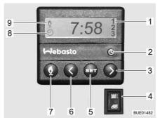
Fig. 213 Operating unit for independent vehicle heater
