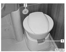
Fig. 285 Toilet bowl with control and operating unit
