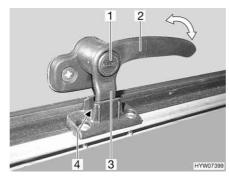
Fig. 76 Catch lever with safety knob in "continuous ventilation" position
