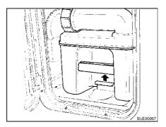
Fig. 268 Pulling the retaining clip
