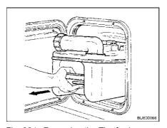
Fig. 264 Removing the Thetford cassette
