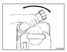
Fig. 254 Turning drainage neck
