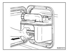
Fig. 253 Removing the Thetford cassette
