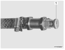
Fig. 290 Bleeding valve of hot-water heater
