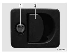
Fig. 47 Flap lock with recessed handle
