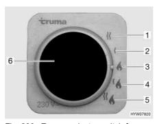
Fig. 200 Energy selector switch for heater/boiler
