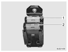
Fig. 186 Fuses for fuel cell
