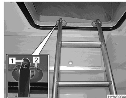
Fig. 83 Access ladder (attached)
