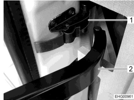
Fig. 16 Limiting lever (Delfin C)
