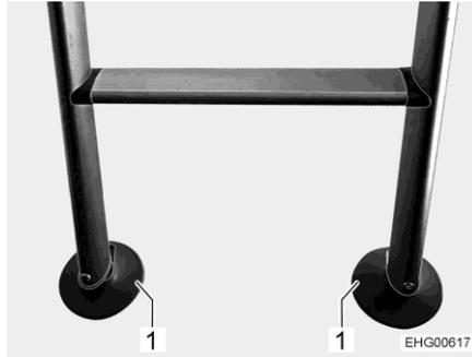
Fig. 84 Plastic plate on the access ladder
