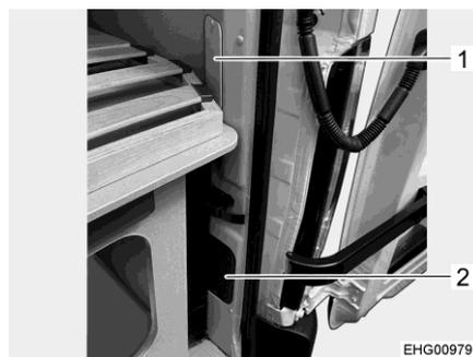
Fig. 138 Access to the fixture of the rear lights unit (Delfin C)
