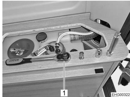
Fig. 137 Access to the fixture of the rear lights unit (Campeo/Eliseo)
