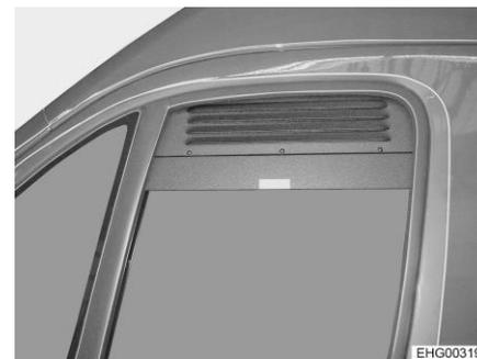
Fig. 79 Forced ventilation grille (side window closed)
