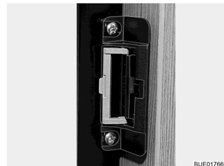
Fig. 117 Locking device in ventilation position
