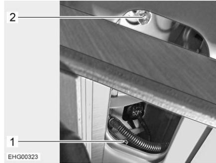
Fig. 139 Fixture of the rear lights unit
