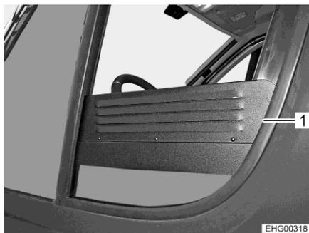
Fig. 78 Forced ventilation grille (side window open)
