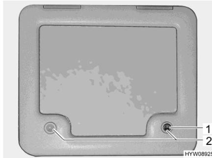
Fig. 133 Flap for the sewage tank
