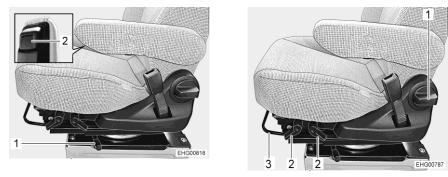
Fig. 16 Release lever for rotating
