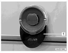
Fig. 9 Flue shield
