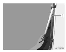
Fig. 79 Hinged window with rotary hinge
