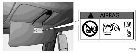
Fig. 15 Warning notice on child restraint system (front passenger's seat sun visor)
