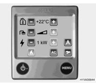
Fig. 130 Adjustment menu (operating unit)
