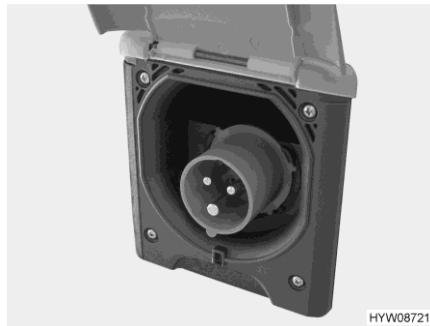
Fig. 48 230 V connection on the vehicle (CEE socket outlet)
