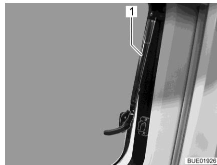
Fig. 13 Hinged window with automatic hinges, open
