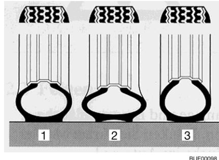
Fig. 83 Contact surface of the tyre
