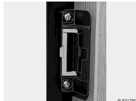
Fig. 64 Locking device in ventilation position
