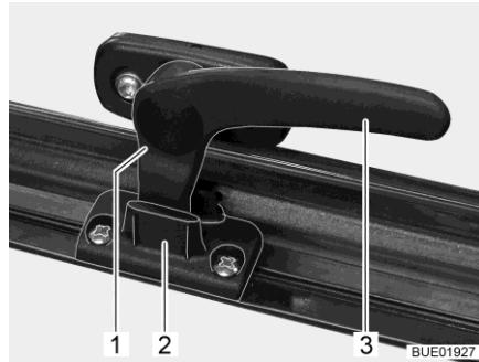
Fig. 14 Catch lever in "continuous ventilation" position
