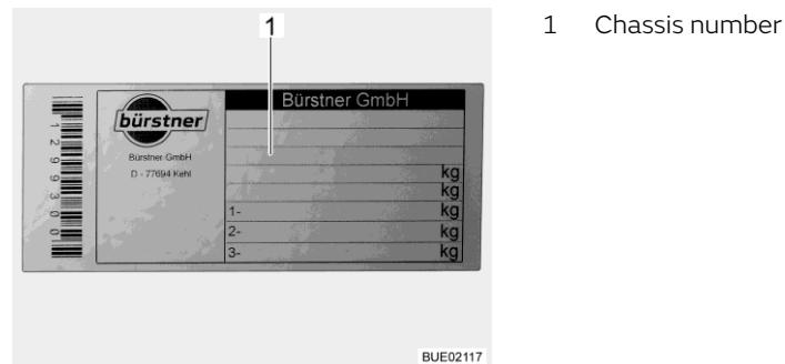
Fig. 81 Vehicle identification plate
