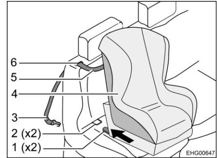
Fig. 7      Fastening with top tether
