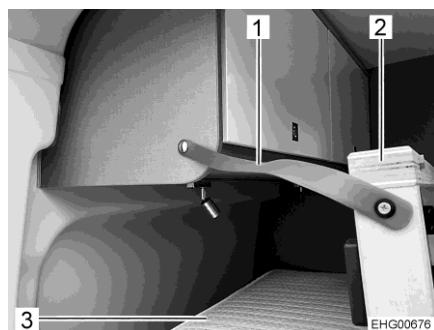
Fig. 35 Bed base retaining strap
