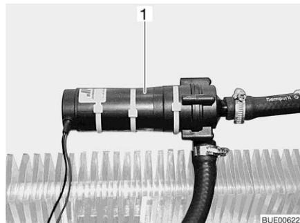
Fig. 143 Auxiliary circulating pump
