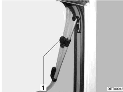
Fig. 70 Hinged window with rotary hinge
