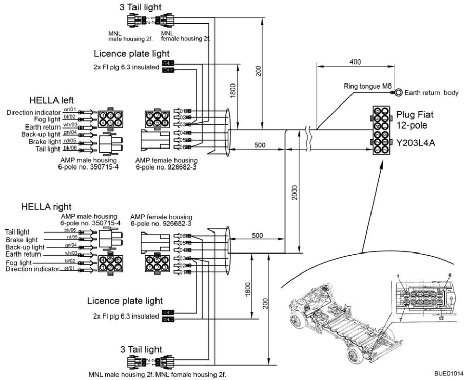
Fig. 135 Circuit diagram, exterior
