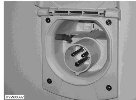
Fig. 123 230 V connection on the vehicle
