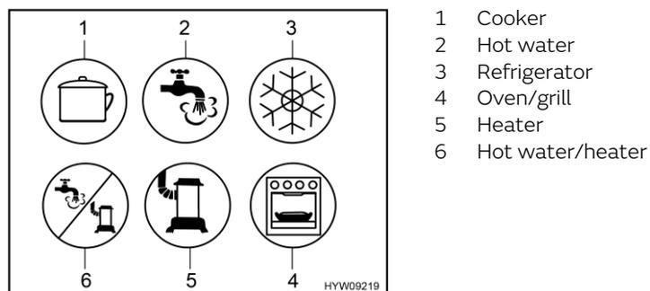
Fig. 136 Possible symbols for the gas isolator taps
