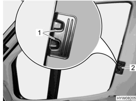
Fig. 24 Roman shade for the driver's / front passenger's window
