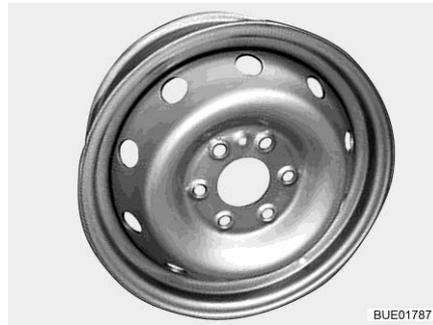
Fig. 199 Steel wheel rim (standard)
