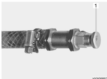
Fig. 187 Bleeding valve of hot-water heater
