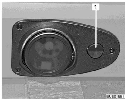
Fig. 59 Recessed LED light, light switch directly on the lamp
