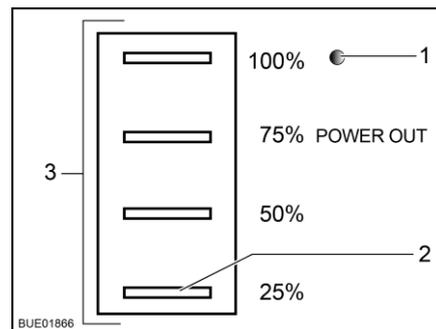
Fig. 121 Status indicator, solar charge regulator
