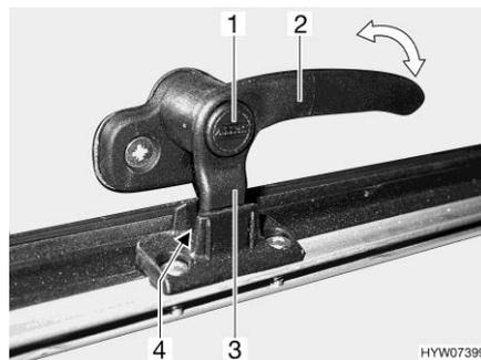
Fig. 72 Catch lever with safety knob in "continuous ventilation" position
