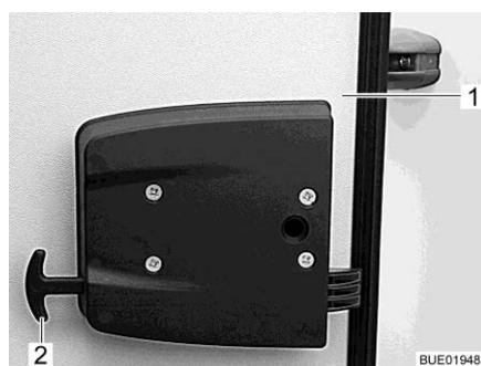
Fig. 40 Garage flap emergency release
