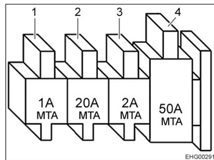
Fig. 127 Fuses (living area battery with charging booster)
