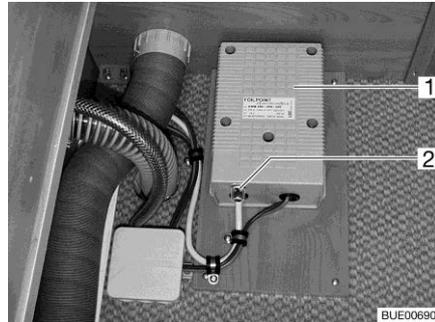
Fig. 147 Transformer for electrical floor warming unit
