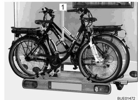
Fig. 5 Positioning of e-bikes
