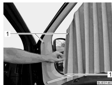
Fig. 77 Fixing of pleated shades
