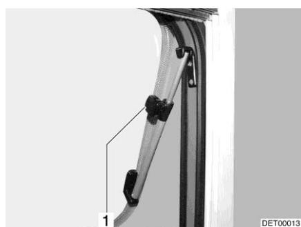
Fig. 90 Skylight with rotary hinges, open
