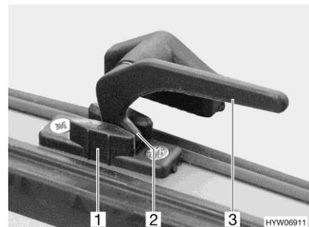
Fig. 73 Catch lever in "continuous ventilation" position
