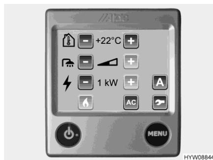
Fig. 139 Adjustment menu (operating unit)
