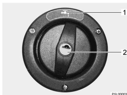
Fig. 45 Cap for the drinking water filler neck
