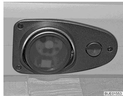
Fig. 193 LED light with switch
