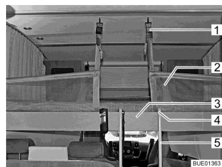
Fig. 123 Pull-down bed complete with applied safety net
