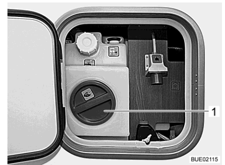
Afb. 307 Reinigingsopening watertank (service-unit)
