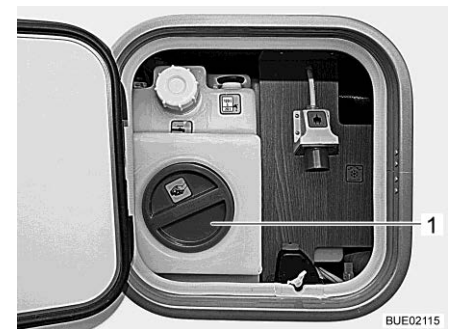
Afb. 303 Reinigingsopening watertank (service-unit)
