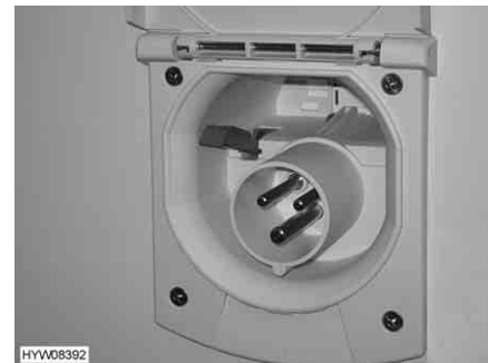
Fig. 121 230 V connection on vehicle
