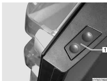
Fig. 158 Release button (refrigerator door, Dometic 8 series)
