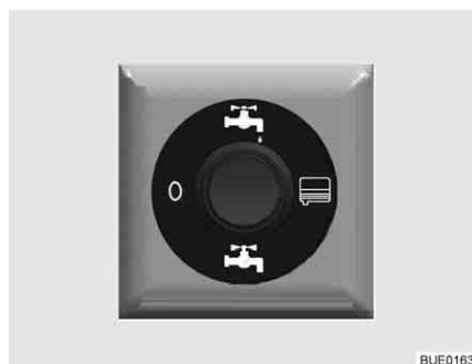
Fig. 170 Operating switch for electrically operated drainage valve
