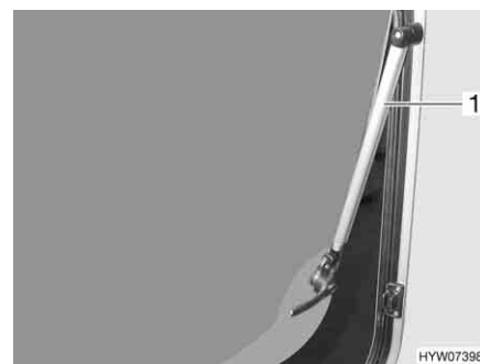
Fig. 69 Hinged window with automatic hinge
