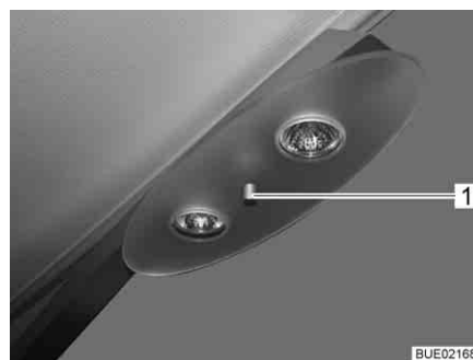
Fig. 55 Spotlight, switch mounted directly on the lamp
