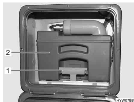
Fig. 174 Sewage tank (example)
