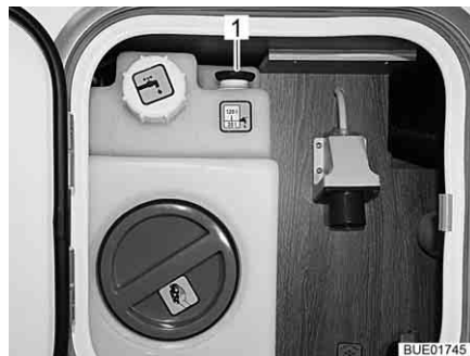
Fig. 243 Water tank (central supply unit)
