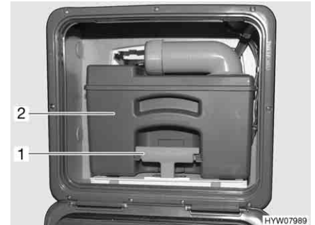
Fig. 253 Sewage tank (example)
