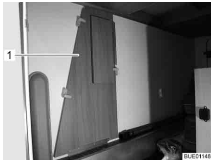
Fig. 13 Bed widening in the rear garage
