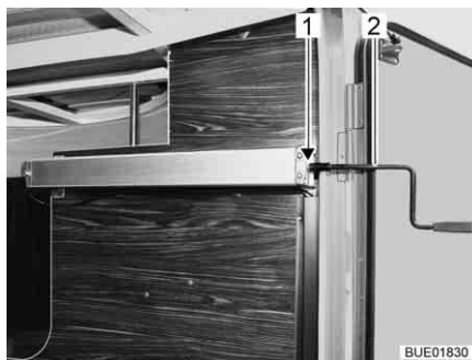
Afb. 118 Handslinger in garage achter
