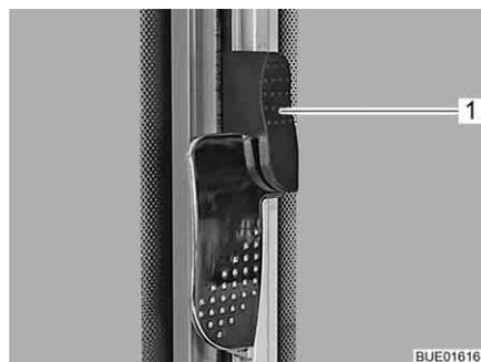
Fig. 108 Sliding window with swivel lock (locked)
