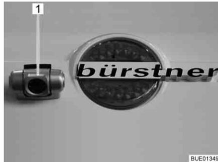
Fig. 19 Reversing camera with infrared illumination
