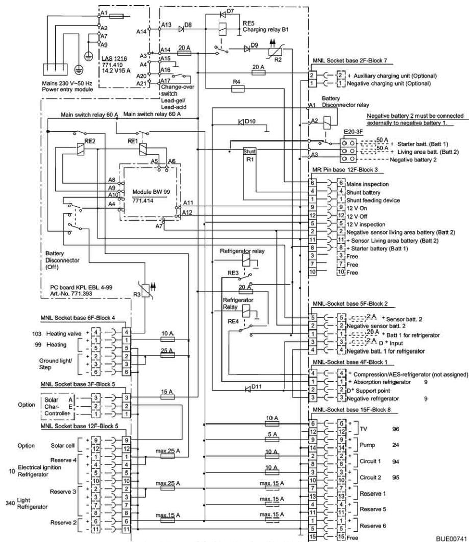
Fig. 172 Circuit diagram, interior (EBL 99)
