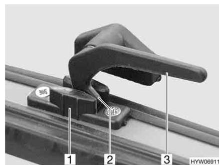
Fig. 106 Catch lever in "continuous ventilation" position
