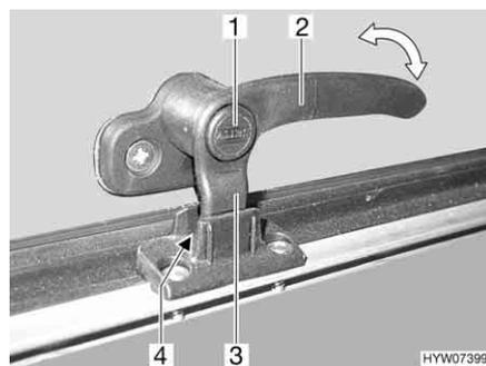
Fig. 105 Catch lever with safety knob in "continuous ventilation" position
