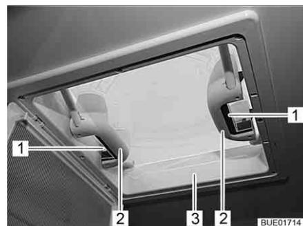
Fig. 121 Handles with snap latches
