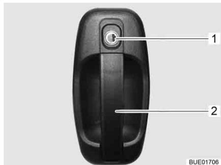
Fig. 63 Door lock of conversion door, outside
