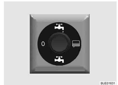
Fig. 231 Operating switch for electrically operated drainage valve (partially special equipment)
