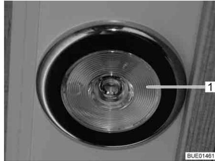
Fig. 90 Recessed light, light switch in the lamp
