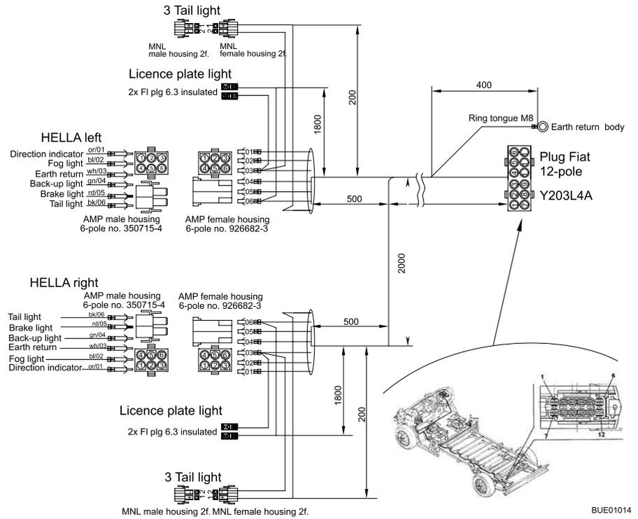
Fig. 176 Circuit diagram, exterior
