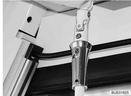
Fig. 115 Journal with attached hand crank
