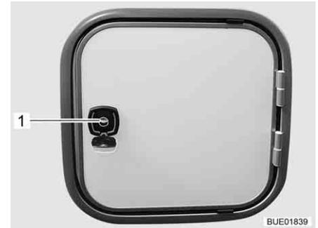
Fig. 245 Flap for sewage tank (alternative)
