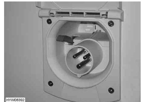
Fig. 162 230 V connection on vehicle
