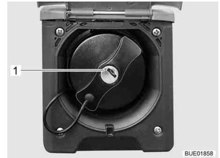
Fig. 47 Cap for the fuel filler neck
