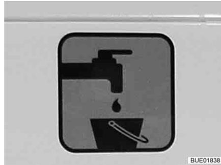
Fig. 229 Drain pipe symbol
