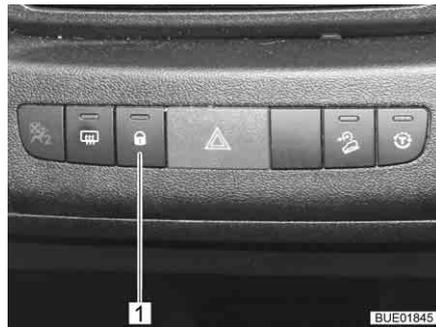
Fig. 59 Switch for the central locking system (Elegance)
