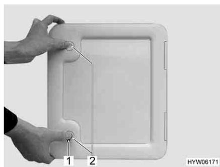
Fig. 235 Flap for sewage tank
