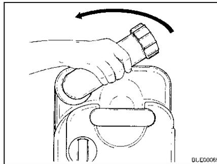
Fig. 238 Turning drainage neck
