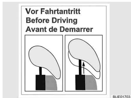
Fig. 30 Symbol "Adjust headrests"
