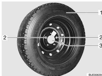
Fig. 276 Spare wheel support in the rear garage
