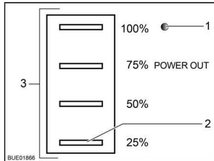
Fig. 160 Status indicator, solar charge regulator
