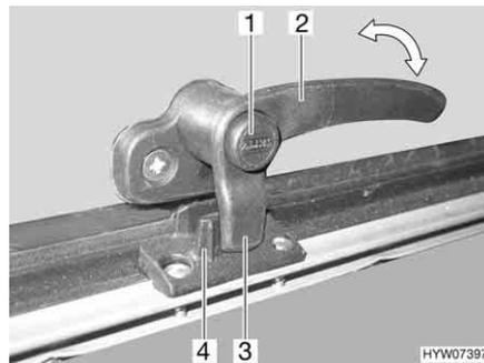
Fig. 101 Catch lever with safety knob in "closed" position
