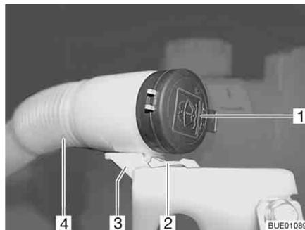
Fig. 43 Washer fluid container filler neck
