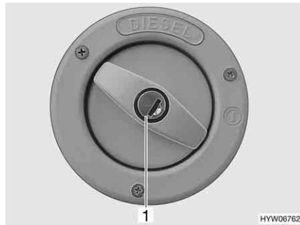
Fig. 45 Cap for the fuel filler neck
