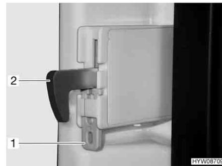
Fig. 212 Lock hook fixture
