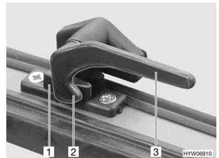
Fig. 102 Catch lever in "closed" position
