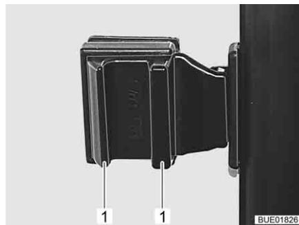
Fig. 107 Sliding window with pressure lock
