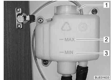
Fig. 252 Compensator reservoir without panel
