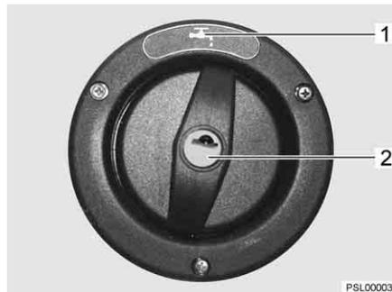
Fig. 218 Cap for the drinking water filler neck
