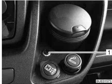
Fig. 53 Push-button to activate remote control
