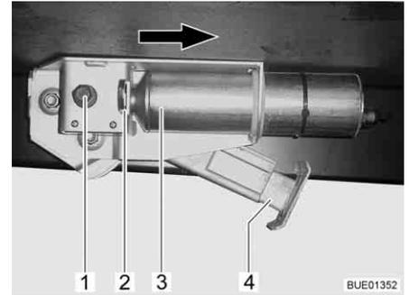
Fig. 54 Electrical steady leg on vehicle
