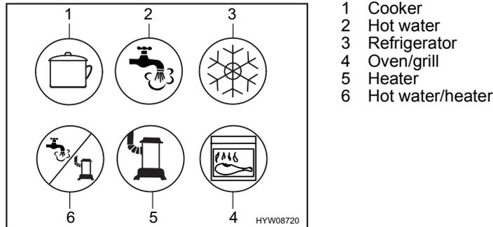
Fig. 147 Possible symbols for the gas isolator taps
