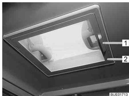
Fig. 120 Skylight with snap latch
