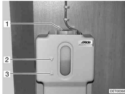
Fig. 251 Compensator reservoir with panel
