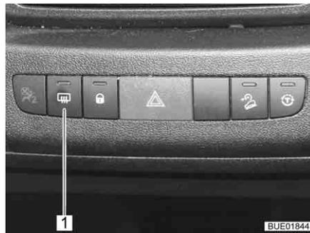
Fig. 36 Switch for the external mirror heater (Elegance)
