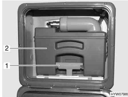
Fig. 237 Sewage tank (example)
