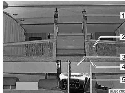
Fig. 139 Pull-down bed complete with applied safety net
