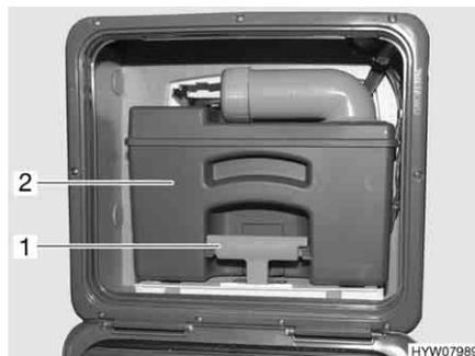
Fig. 246 Sewage tank (example)
