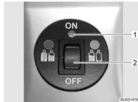
Fig. 152 Operating unit with remote display
