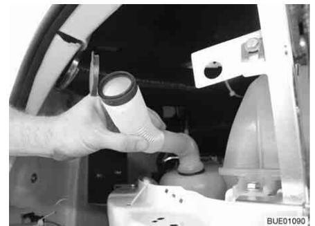
Fig. 44 Filler neck in filling position
