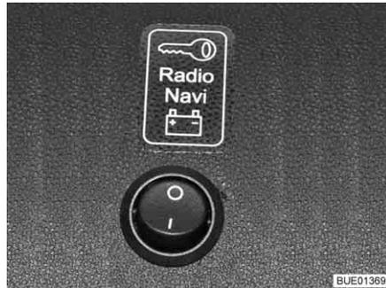
Fig. 151 Selector switch for operating behaviour
