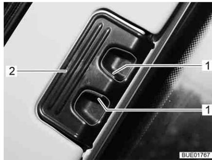
Fig. 110 Locking mechanism for driver's/front passenger's windows
