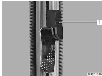
Fig. 103 Sliding window with swivel lock (locked)
