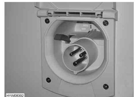
Fig. 164 230 V connection on vehicle
