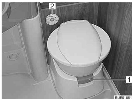
Fig. 261 Toilet bowl with control and operating unit
