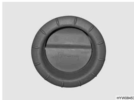
Fig. 187 Air outlet nozzle of the hot air distribution
