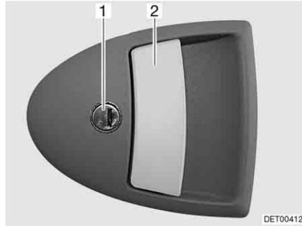
Fig. 57 Door lock of conversion door, outside
