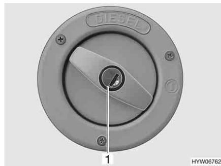
Fig. 43 Cap for the fuel filler neck
