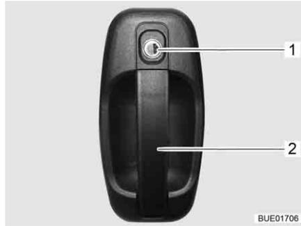
Fig. 55 Door lock of conversion door, outside
