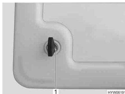
Fig. 64 Push-button lock service flap
