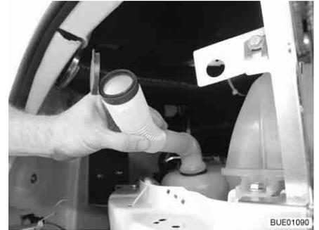
Fig. 42 Filler neck in filling position
