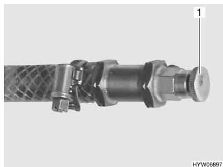
Fig. 270 Bleeding valve of hot-water heater
