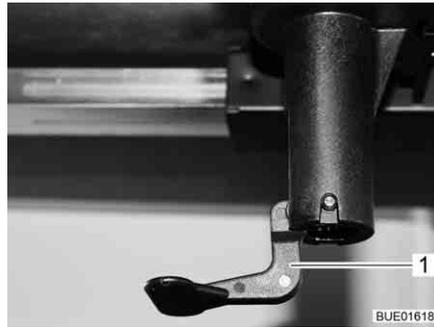
Fig. 118 Unlocking of the table top
