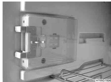
Fig. 234 Locking device in ventilation position
