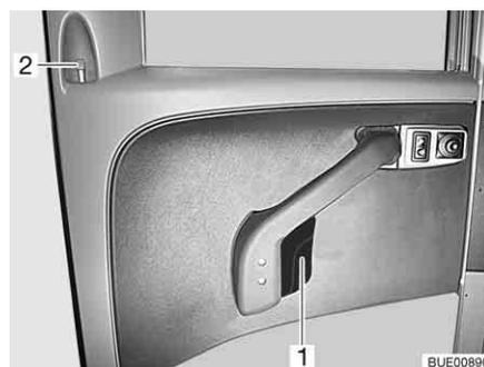
Fig. 54 Door lock of driver's door, inside
