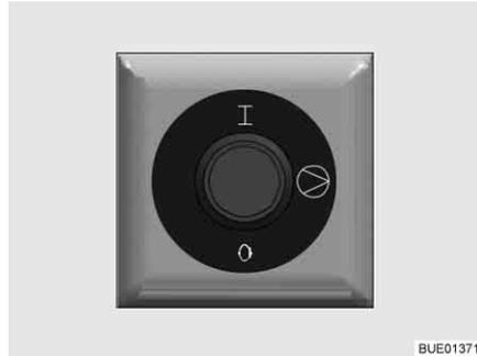
Fig. 200 Operating switch for auxiliary circulating pump
