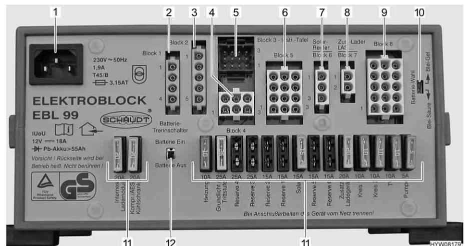
Fig. 105 Transformer/rectifier (EBL 99)
