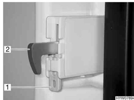
Fig. 146 Lock hook fixture
