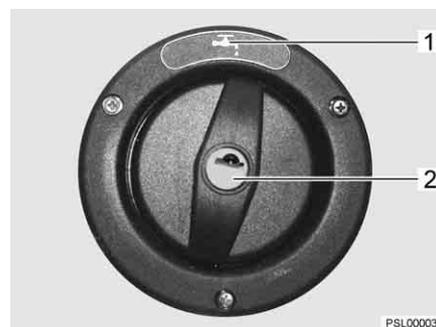
Fig. 40 Cap for the drinking water filler neck
