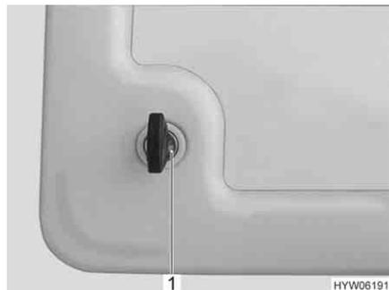
Fig. 38 Push-button lock service flap
