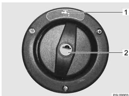
Fig. 149 Cap for the drinking water filler neck
