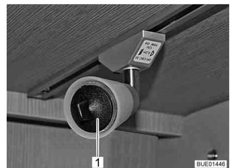
Fig. 181 Suction cup for replacing the lamp
