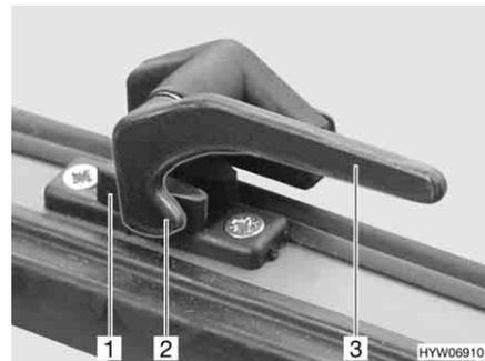
Fig. 53 Catch lever in "closed" position
