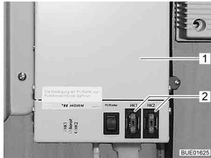
Fig. 116 Heater regulation for waste water pipes
