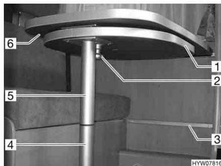
Fig. 79 Suspension table with separable support leg
