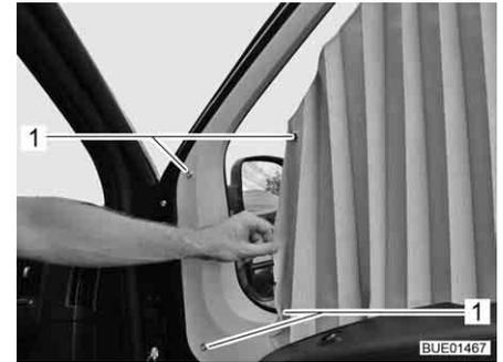
Fig. 64 Fixing of pleated shades
