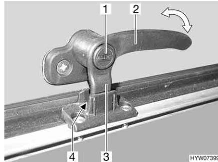
Fig. 55 Catch lever with safety knob in "continuous ventilation" position
