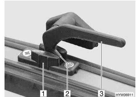
Fig. 56 Catch lever in the "continuous ventilation" position
