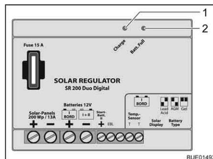
Fig. 108 Solar charge regulator 200 W
