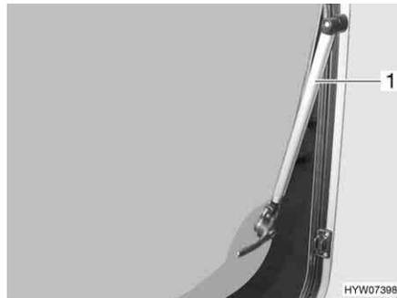
Fig. 59 Hinged window with automatic hinges
