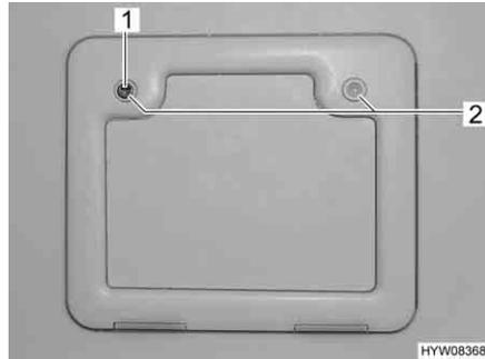
Fig. 172 Flap for the sewage tank
