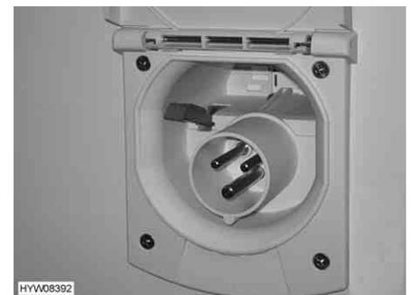
Fig. 110 230 V connection on vehicle
