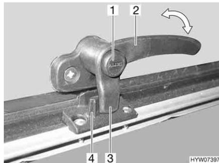
Fig. 52 Catch lever with safety knob in "closed" position
