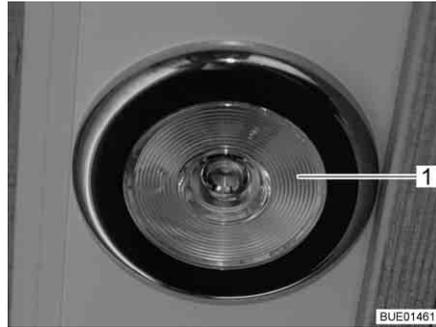
Fig. 47 Recessed light, light switch in the lamp
