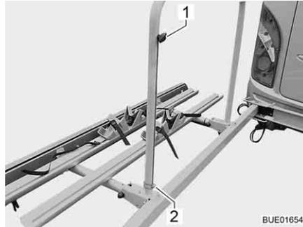
Fig. 3 Securing the support
