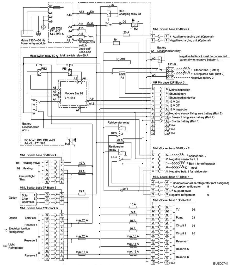
Fig. 123 Circuit diagram, interior (EBL 99)
