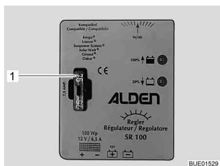
Billede 182 Sikring solcelleladeregulator 100 W
