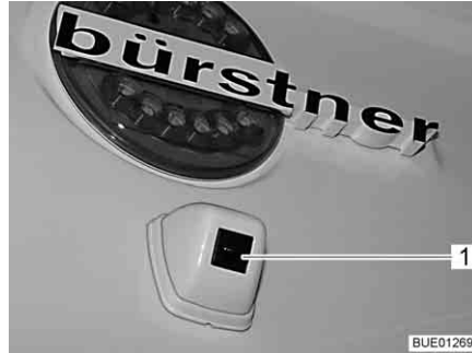
Fig. 21 Telecamera retromarcia (Pioneer)
