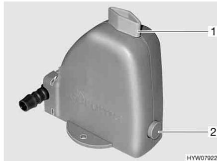
Fig. 149 Safety/drainage valve of the boiler
