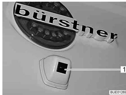
Fig. 16 Reversing camera (example)
