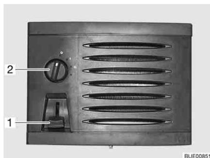
Fig. 140 Operating controls for auxiliary heat exchanger
