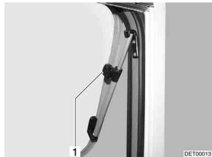
Fig. 71 Skylight with rotary hinges, open
