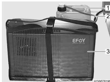
Fig. 109 Fuel cell with tank cartridge
