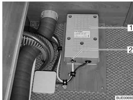
Fig. 141 Transformer for electrical floor warming unit
