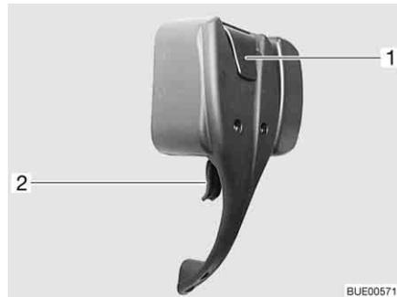
Fig. 28 Door lock of conversion door, inside, locked
