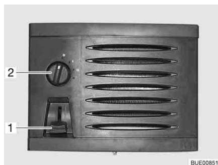
Fig. 172 Operating controls for auxiliary heat exchanger
