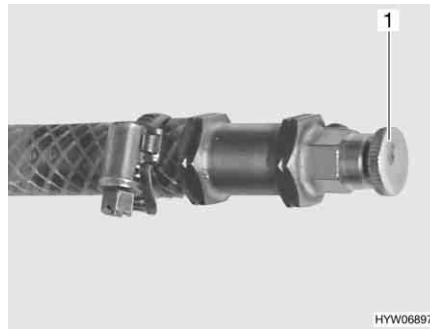
Fig. 253 Bleeding valve of hot-water heater
