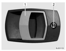
Fig. 31 Door lock of conversion door, outside
