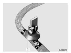
Fig. 225 Drain cock (with rocking lever)
