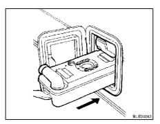
Fig. 233 Inserting the Thetford cassette
