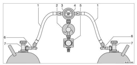
Fig. 145 Crash protection unit switching facility
