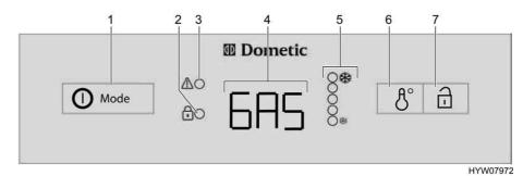
Fig. 210 Operating controls for the refrigerator (Dometic 8 series with AES)
