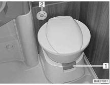
Fig. 262 Toilet bowl with control and operating unit
