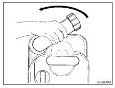
Fig. 247 Turning drainage neck
