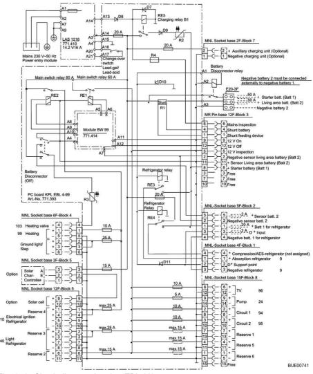
Fig. 171 Circuit diagram, interior (EBL 99)
