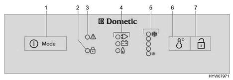
Fig. 209 Operating controls for the refrigerator (Dometic 8 series with MES)
