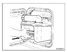
Fig. 257 Inserting the Thetford cassette
