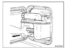
Fig. 254 Removing the Thetford cassette
