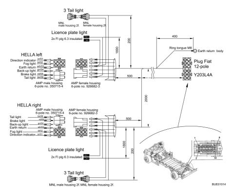
Fig. 174 Circuit diagram, exterior
