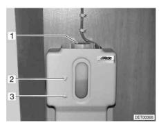
Fig. 267 Compensator reservoir hotwater heater
