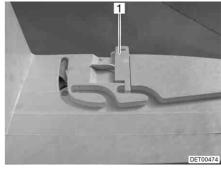
Fig. 70 Ventilation position locking mechanism
