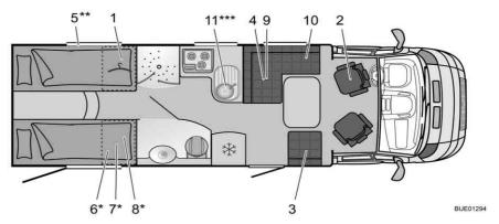
Fig. 308 Ground plan T 728 Nexxo
