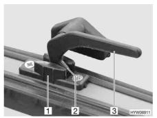
Fig. 58 Catch lever in the "continuous ventilation" position
