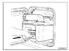
Fig. 244 Inserting the Thetford cassette
