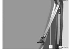
Fig. 59 Catch lever in "closed" position
