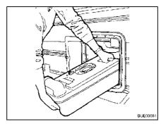
Fig. 230 Removing the Thetford cassette
