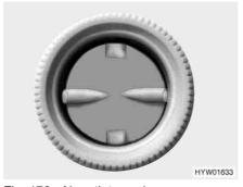
Fig. 176 Air outlet nozzle
