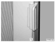
Fig. 23 Locking mechanism for Roman shade on driver's/front passenger's windows
