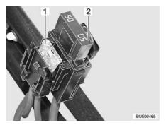
Fig. 160 Fuses on the starter battery
