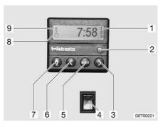
Fig. 188 Operating unit for independent vehicle heater
