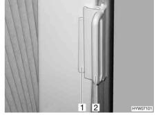
Fig. 66 Roman shades for driver's window and front passenger's window
