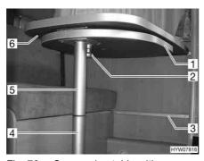
Fig. 76 Suspension table with separable support leg
