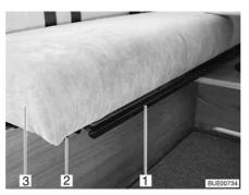
Fig. 20 Backrest adjustment mechanism for bench
