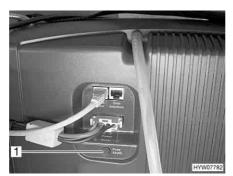
1 Safety fuse 250 V 8.0 A M (medium delayed-action) 20 x 5 mm
