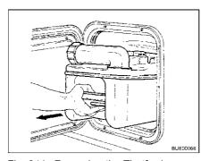
Fig. 241 Removing the Thetford cassette
