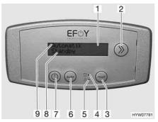
Fig. 155 Operating unit fuel cell
