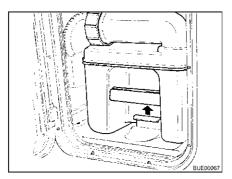
Fig. 245 Pulling the retaining clip
