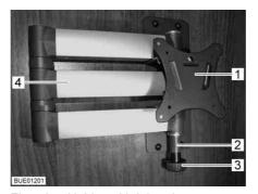
Fig. 52 Holder with jointed arm
