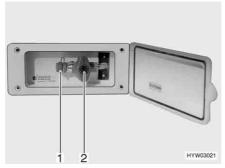
Fig. 144 External gas connection, gas isolator tap closed
