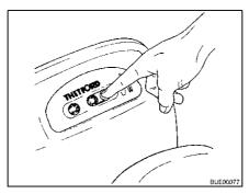
Fig. 240 Closing the sliding trap
