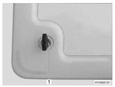
Fig. 36 Push-button lock service flap
