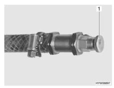
Fig. 268 Bleeding valve of hot-water heater
