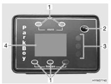
Fig. 15 Parking distance control operating unit
