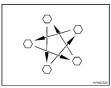
Fig. 282 Tighten the wheel nuts or wheel bolts cross-wise
