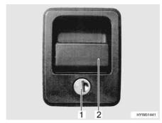
Fig. 35 Flap lock with recessed handle
