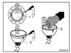
Fig. 273 Recessed halogen light (flat)
