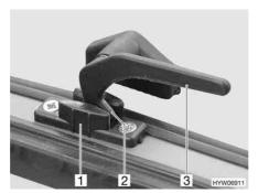
Fig. 61 Catch lever in the "continuous ventilation" position
