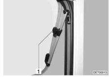
Fig. 72 Catch lever in "closed" position
