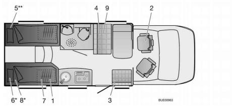
Fig. 291 Ground plan T 620 Travel Van
