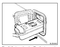
Fig. 249 Inserting the Thetford cassette
